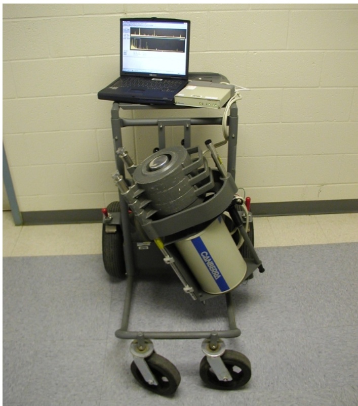
Exhibit 4-11: ISOCS Portable Gamma Spectroscopy System.
