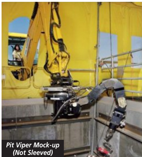
Exhibit 4-2: Pit Viper Robotic Device.
