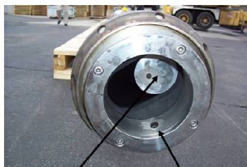
Pump Rotor Dilution Water Supply Port
