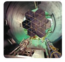
Vacuum Facility 6 (VF6) is a 25-foot-diameter thermal vacuum facility located at NASA Glenn Research Center in Cleveland, Ohio. The test chamber and supporting infrastructure continue to serve as a valuable resource in space environmental ground testing. Some unique facility capabilities include a large chamber volume (25 feet in diameter by 70 feet long), as well as the use of a liquid-nitrogen-cooled shroud and a solar simulator specifically designed for solar-concentrated power.
