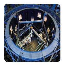
Thermal Vacuum Chamber B, with roughly one-tenth of the internal volume of Chamber A, can handle a variety of smaller-scale tests more economically and with faster response. It is a human-rated chamber equipped with a traversing monorail that provides weight relief to one suited crewmember at a time. The traversing monorail allows two degrees of freedom inside the chamber and 200 square feet (18.6 square meters) of working space.
