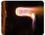
Four individual test facilities, supported by common electrical, vacuum, and cooling systems, comprise the Arc Jet Complex. Premixed air, heated to extreme temperature by a high-power DC discharge, expands through user-selected conical, semi-elliptical, and channel nozzles to hypersonic velocities with enthalpies similar to those experienced by the entry vehicle.
