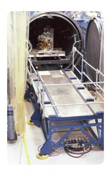
Facility 225 at the Goddard Space Flight Center is a horizontal loading thermal vacuum test chamber used for thermal vacuum and thermal balance testing, as well as for the bakeout of large test items. Electrical feedthroughs and liquid and gas penetrations are provided on the front, sides, and rear of the chamber. A clean tent covering the door opening provides a class 10,000 clean area for integrating hardware prior to loading it into the chamber.
