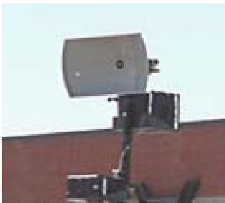
The motion-activated RDTS is used to detect and assess threats at long distances (up to 10 km for vehicles).
