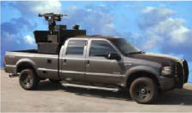
The Advanced Concept Armored Vehicle (ACAV) II with a remotely operated M-240 serves as a force multiplier and enhances survivability.
