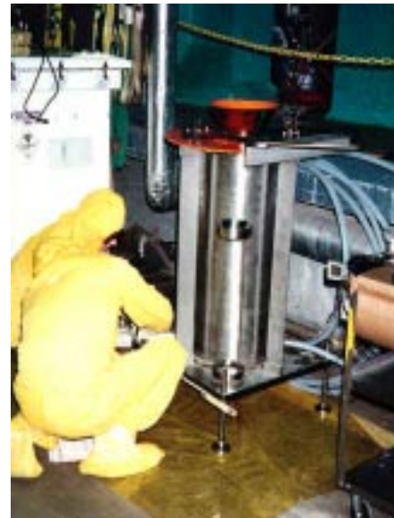
Calibrating Equipment for Measuring Irradiated Fuel
