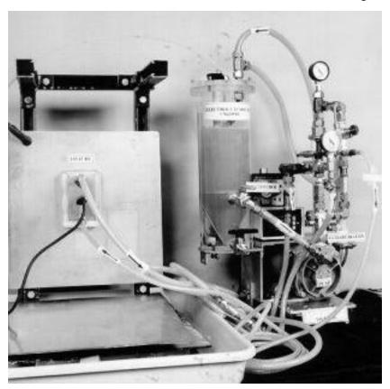
enables material reuse or recycle. Decontamination at the source reduces exposure risks to workers, public and environment in subsequent discard operations. An in-situ plutonium glovebox decontamination method performs a rapid, uniform electrolytic etch of the metal surface, resulting in the removal of the surface contamination. Solution recycle eliminates aqueous process wastes. This technology has been successfully demonstrated during fiscal 1998 and 1999 toward routine implementation.
