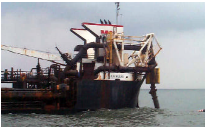
Sand is dredged from the bottom of the ocean and pumped onto Assateague Island. (Photo by Doug Garman)
