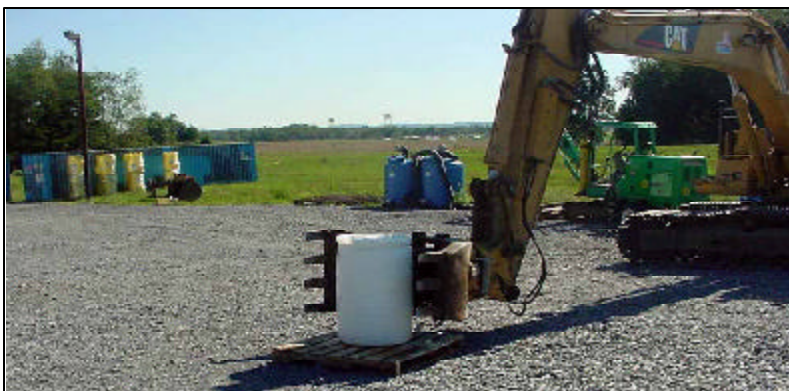
A drum is safely moved with the drum grapppler attachment for a backhoe. (Courtesy U.S. Army COE)
