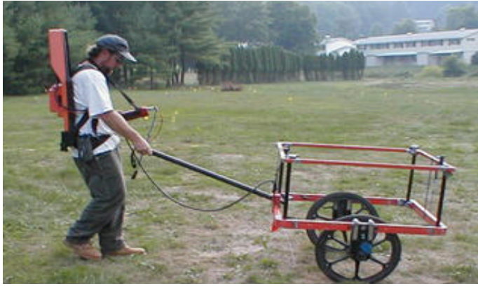
A worker uses an EM-61, electromagnetic induction system, to identify anomalies as deep as three meters below ground.
