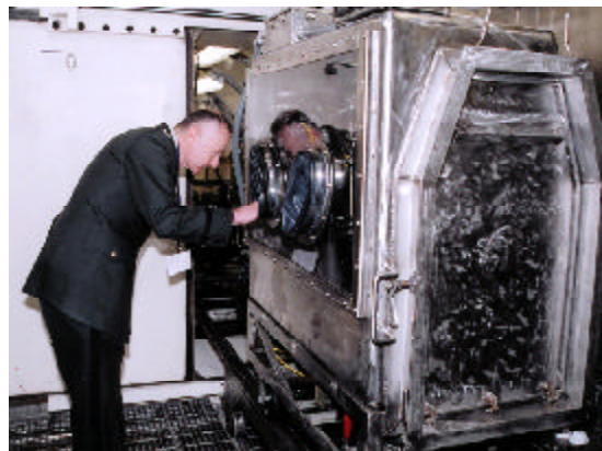
Baltimore District Commander Col. Robert J. Davis inspects the state-of-the-art drill cart at the new MAPS facility. Munitions are moved into an explosive containment chamber and remotely cut and drilled. Photo by Tex Jobe
