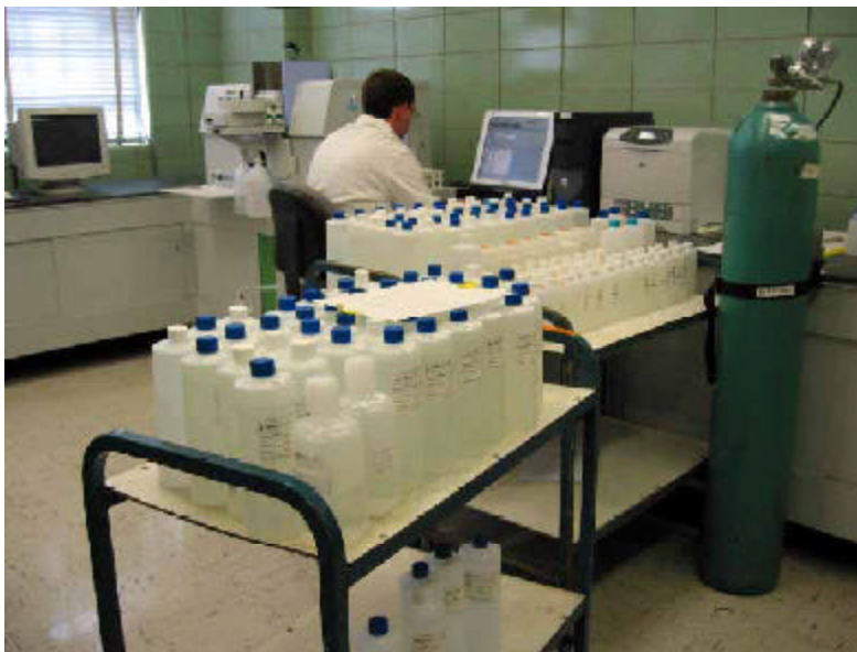
Brett Moody, a Washington Aqueduct employee, uses an atomic absorption analyzer to test for lead in the water. The containers in front are to be tested. (Photo by Elizabeth Turner)
