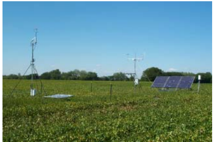
An Eddy Flux tower, powered by solar energy, located at a soybean field at Fermilab is measuring the exchange of carbon dioxide between plants and soil and the atmosphere to study the carbon balance of agricultural fields typical of the U.S. Midwest.
