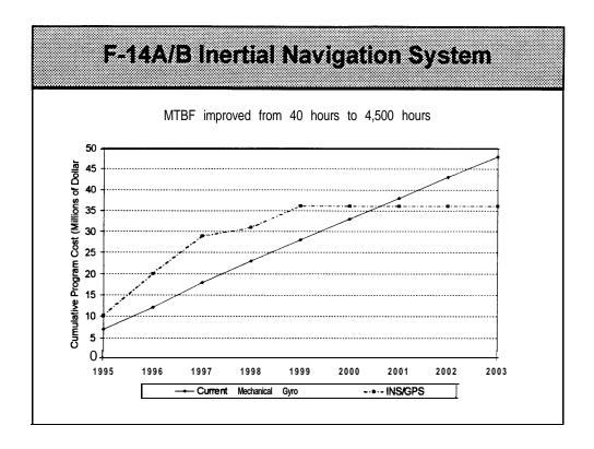
This example of technology insertion for reliability enhancement involves the inertial system on the Navy F-14A/B aircraft. It is based on data provided by the Navy Aviation Supply Office BOSS III program.
