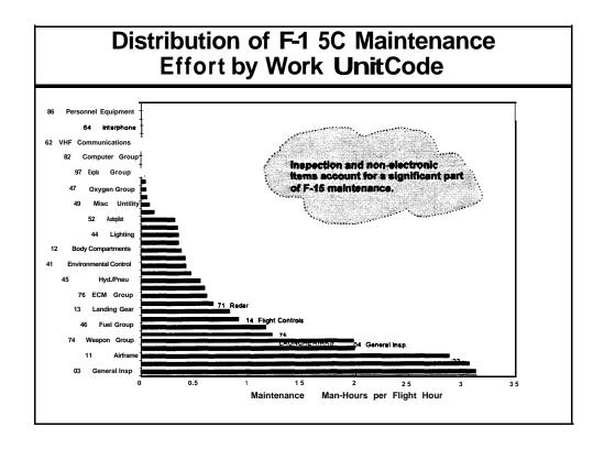
This chart shows how maintenance man-hours per flight hour-one surrogate for O&S expenditures--æ distributed for the F-15C aircraft. Again, a significant portion of funding is concentrated in a relatively small number of systems, thereby providing a focus for initial savings opportunities.
