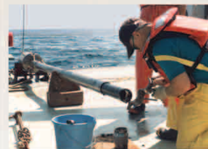
Samples of the sea bottom were taken with two devices. A gravity corer (above) was used where the sediment was expected to be soft and muddy. A clam-like Van Veen grab sampler (left, in closed position), used where the sea floor was expected to be sandy, collected samples such as the sand and brittle stars shown (top).
