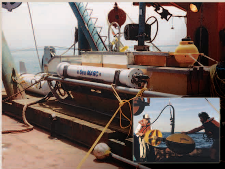
Two types of equipment using sound waves—sidescan sonar and seismic-reflection systems—were used to map the sea floor in the Gulf Of the Farallones. Each system is housed in a hydrodynamic “towfish” that is towed just below the ocean surface from a ship. The SeaMARC1A sidescan-sonar system is shown here outside of its protective shell. The inset shows the towfish that was used for high-resolution seismic-reflection systems.
