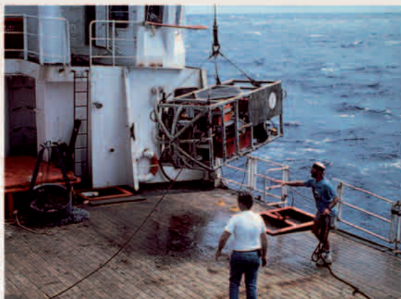
This U.S. Geological Survey camera sled, towed from a research vessel along pre-planned tracklines, was used to take pictures of the sea floor in the Gulf of the Farallones.
