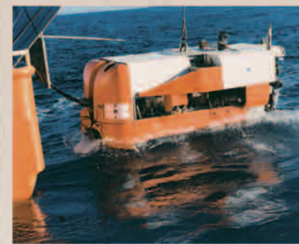
Sea Cliff (above), a manned deep-submergence vehicle operated by the U.S. Navy, was used to directly observe the sea bottom and to take physical samples with its mechanical arms. The Navy’s unmanned Advanced Tethered Vehicle (above right) was also used to take video footage and still photographs of the sea floor.
