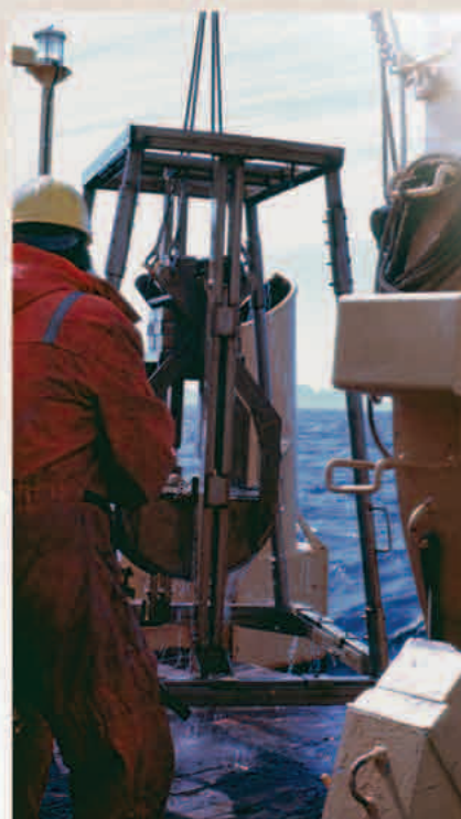
Samples of the sea bottom were taken with two devices. A gravity corer (above) was used where the sediment was expected to be soft and muddy. A clam-like Van Veen grab sampler (left, in closed position), used where the sea floor was expected to be sandy, collected samples such as the sand and brittle stars shown (top).
