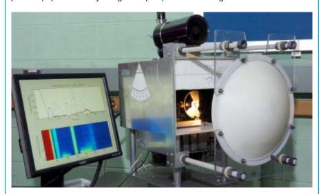
A prototype of the passive millimeter-wave spectroscope.
