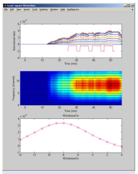
Passive millimeter-wave spectroscopy detection of nitric oxide (NO) plume: (a) normalized signals of hot air and NO for 15 frequency channels, (b) spectral image of the plume, and (c) model-fitted spectral line of NO during its release.
