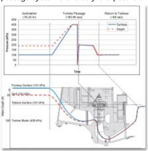
Surface and 30-ft depth pressure exposure simulation of turbine passage.
