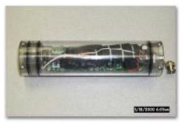
Sensor fish prototype device.
