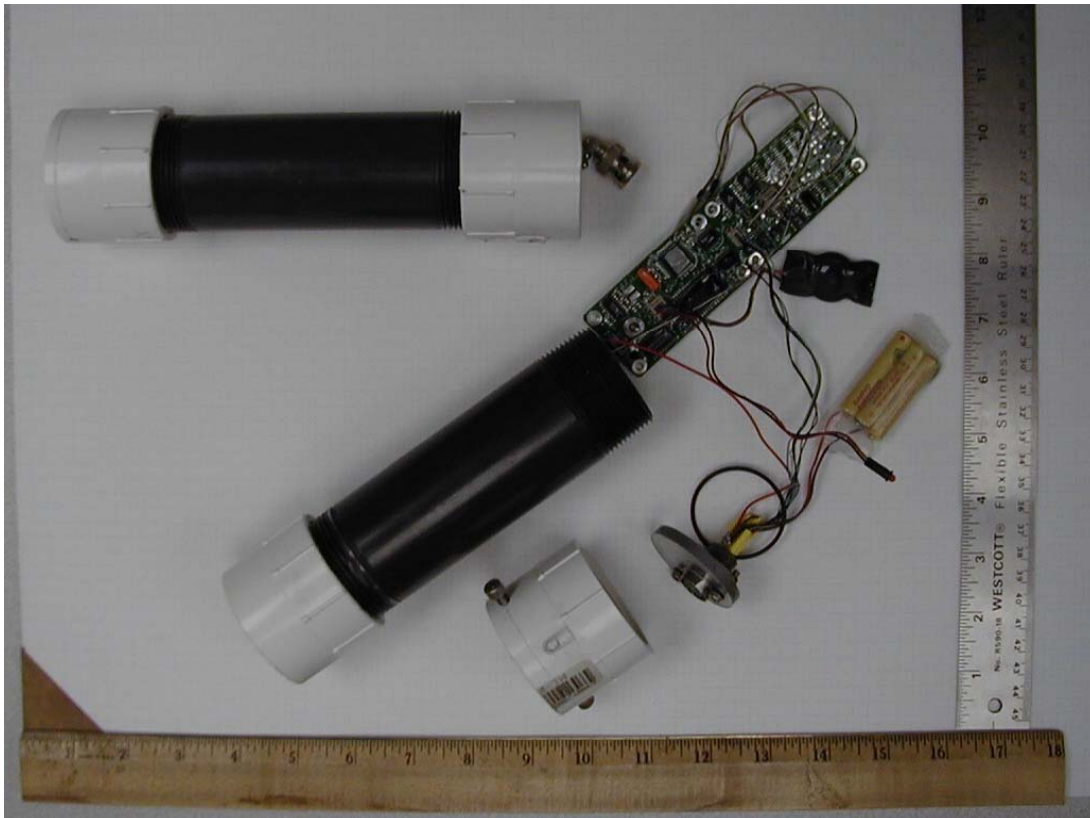
Figure 2.6. Redesigned Sensor Fish Device: PVC Pipe
