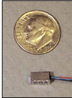
Figure 2.3. Accelerometer Contained in Prototype Sensor Fish Device
