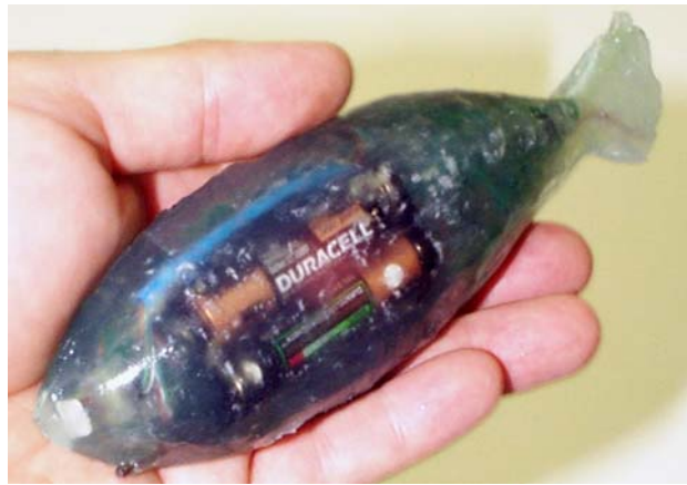
Figure 2.2. Initial Sensor Fish Device
