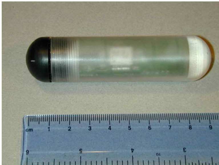
Figure 5.1. New and Improved Sensor Fish Device
