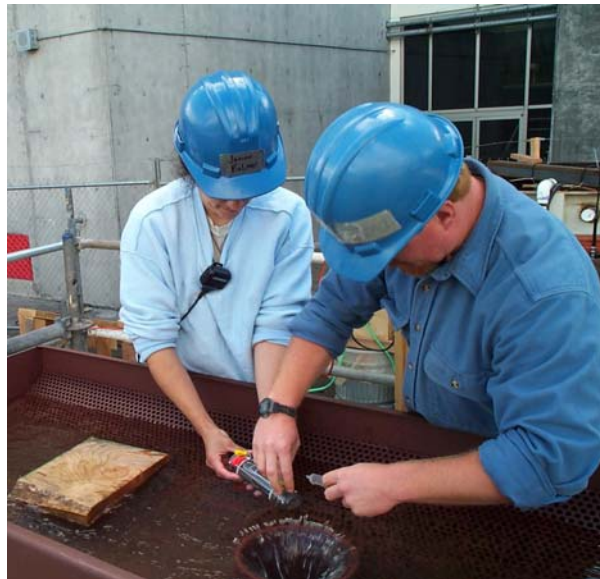
Figure 3.1. Injection System Used to Deploy Sensor Fish
