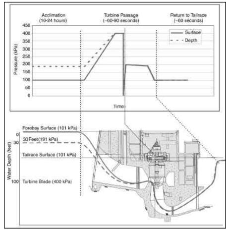
Figure 1: This graph/drawing tracks simulated fish passage through a Kaplan turbine during research conducted by scientists at the Pacific Northwest National Laboratory. Test fish — surface- or depth-acclimated for 16 to 24 hours — move through the turbine in 60 to 90 seconds and into the tailrace in approximately 60 seconds. The upper graph shows the rapid pressure changes the fish undergo.
