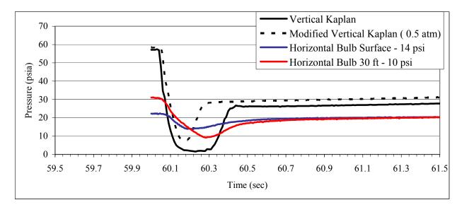
**Figure 2.3**. Comparison of the expected pressure nadirs during passage through a typical vertical Kaplan turbine, a modified vertical Kaplan turbine, and two horizontal bulb turbine passage scenarios.
