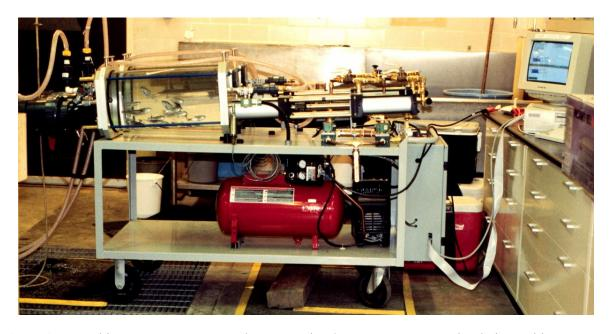
Figure 2.1. Turbine passage system used to create time/pressure sequences simulating turbine passage.
