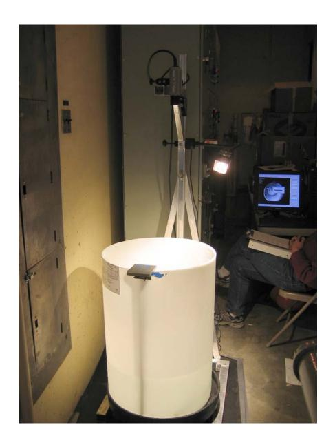
Figure 2.3. C-start filming apparatus used for the Wanapum tests. A high-speed digital video camera recorded movements of fish in the white, 80-cm-high filming tank. The strike plate and rod extending into the water are clamped on the front of the tank. The computer monitor that displayed the video images can be seen in the background.
