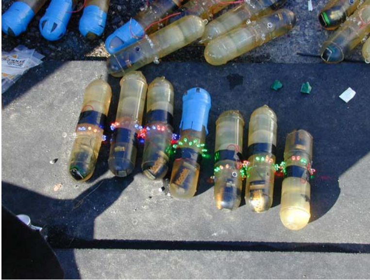
Figure 2. Near neutrally buoyant drogues lighted with different colors of ultrabright light-emitting diodes.
