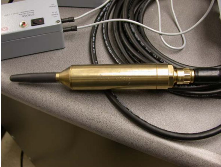
Figure 4. Reson hydrophone used to measure noise.
