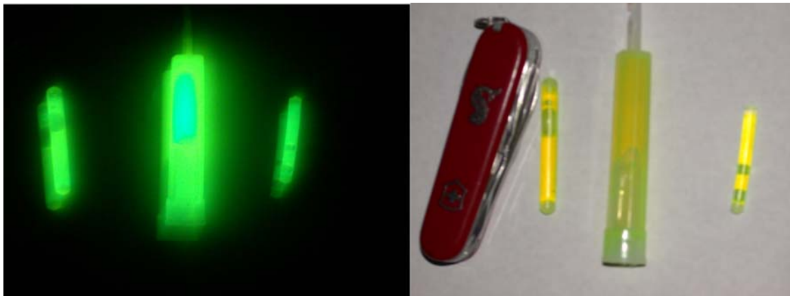
Figure 1. Green (Cyalume Lightsticks™) chemical lightsticks (5.1 cm, 10.2 cm, and 3.8 cm from left to right) used in feasibility testing at Bonneville and McNary Dams and in evaluation of camera tracking arrays. (Studies conducted by PNNL for Portland and Walla Walla District USACE, respectively.)
