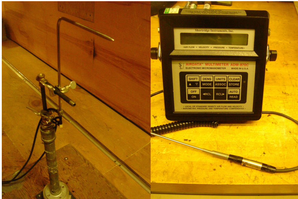
Figure 1. Instrument under test in NIST Wind Tunnel, viewed from upstream and the readout.
