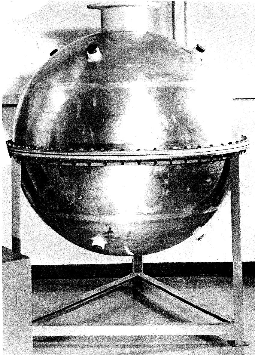
FIG. 3. A photograph of the aluminum shell which supports the polyethylene liner and MnSO_4 solution. Sources are pulled into the center of the solution by a Teflon can attached to a rope on a pulley, above, and a short steel bar at the bottom of the inside of the spherical tank.
