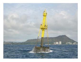
important for most of Europe. As with some of other wave energy conversion models that have been presented, these PowerBuoys have a minimal visual profile and a high power density. We can get one megawatt from an area of 1.6 acres, given suitable wave conditions.
