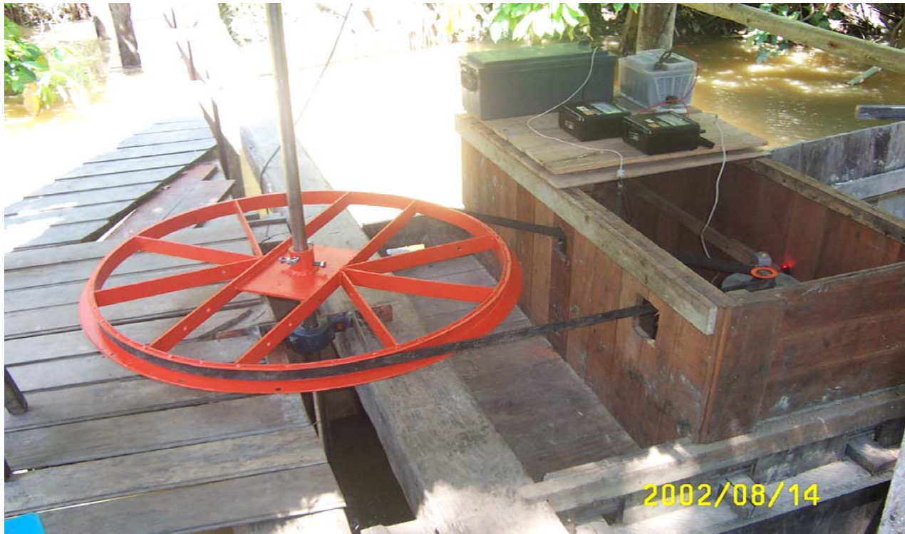
Views of the pulley, belt drive, alternator, monitoring equipment, rheostat, and batteries.
