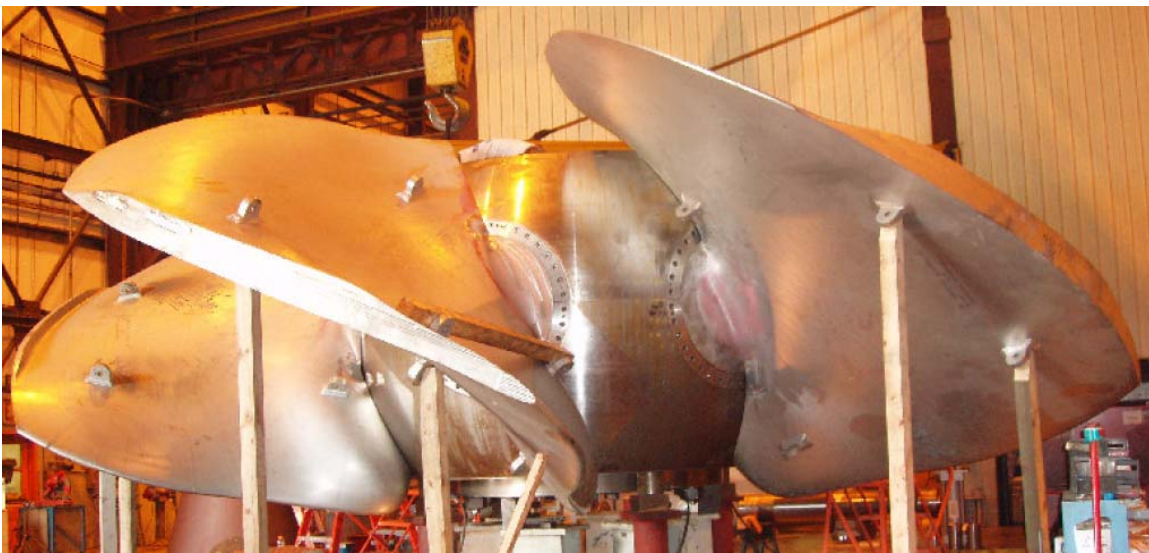
Figure 2.7. Unit 8 (AHT) Runner and Spherical Hub (photo provided by Voith Siemens Hydropower)
