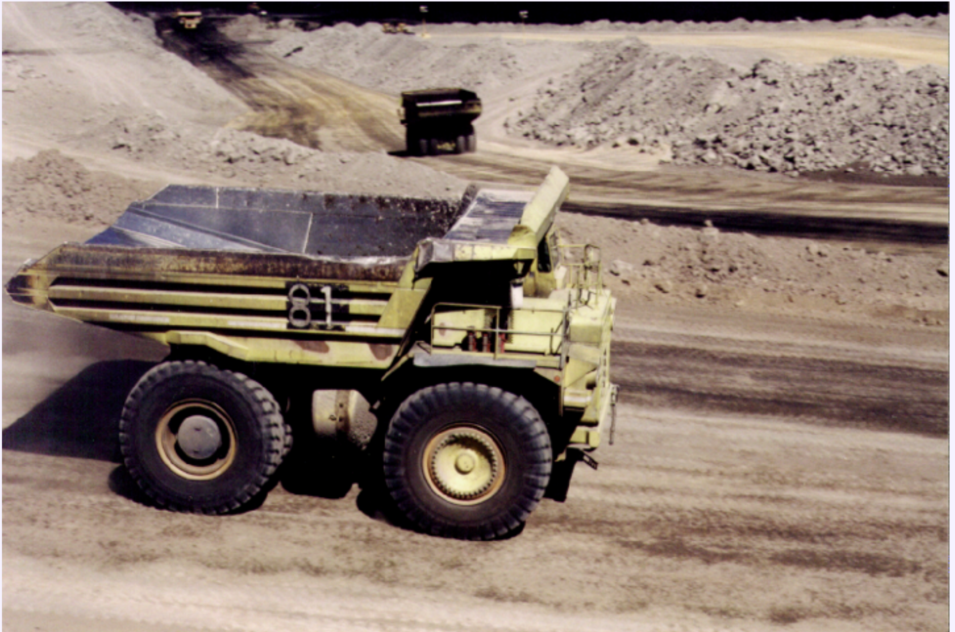
Figure MO-28. This Euclid end-dump truck is returning from the spoil dump to the highwall for another load of overburden.
