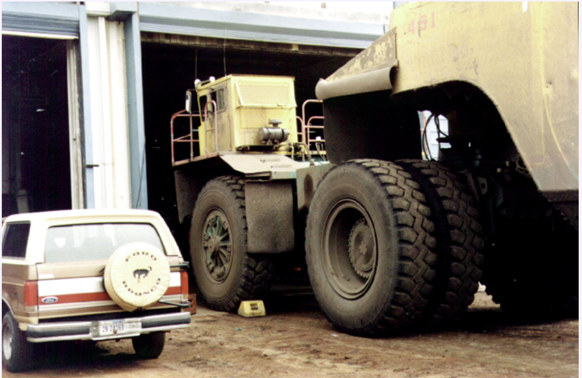
Figure MO-38. Normally, trucks receive preventive maintenance in the field or on the ready line. This 200 ton, tractor-trailer, belly-dump truck is receiving maintenance at the main shop area.
