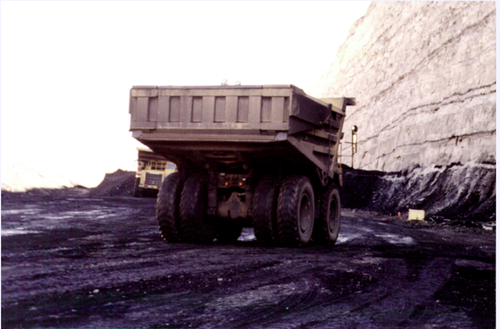
Figure MO-27. Large Caterpillar end-dump trucks are used to haul coal from the coal face to primary crushers at strategic locations above the pit ramps.
