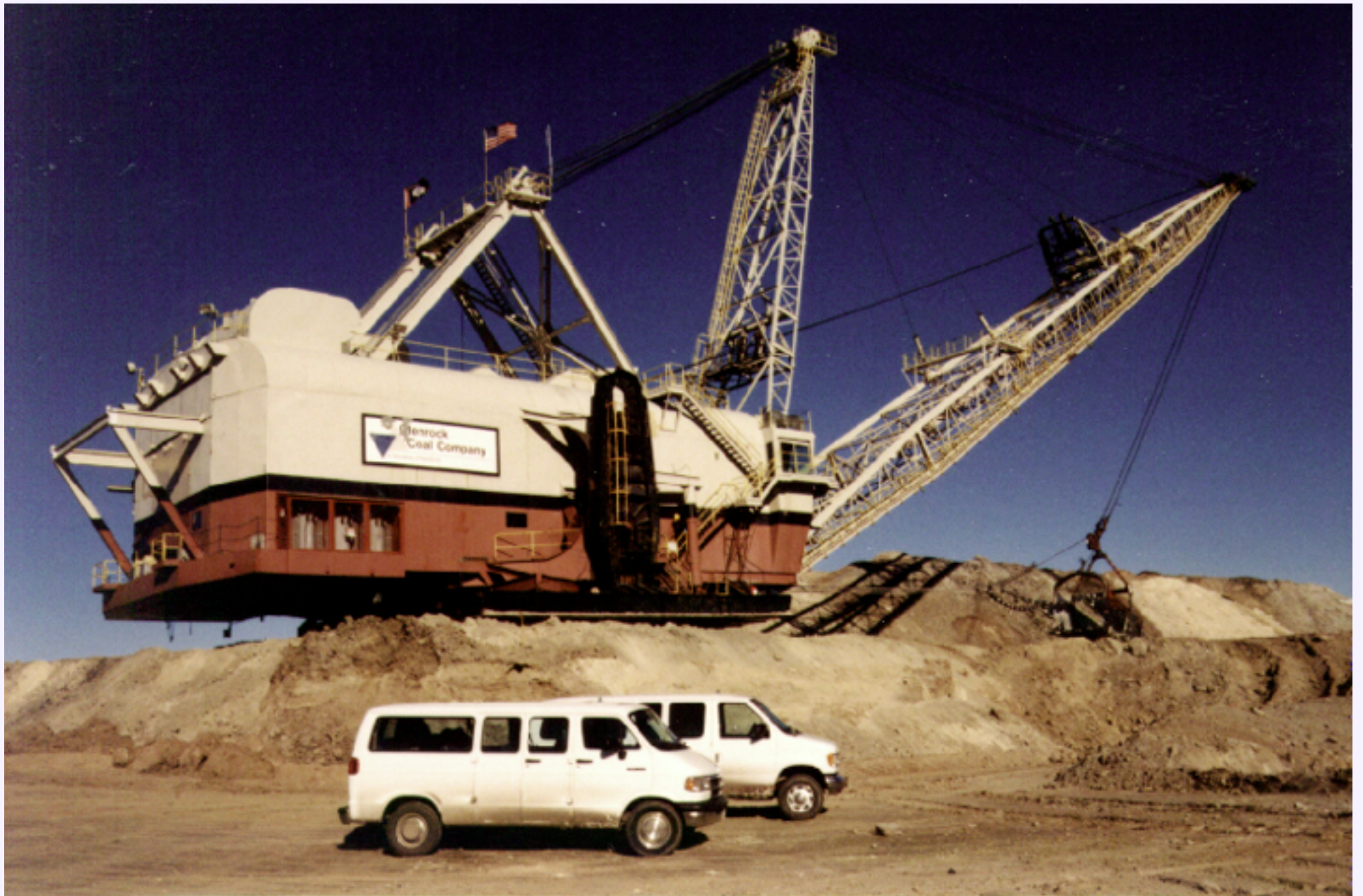
Figure MO-24. A Page 752 dragline with vans in the foreground for scale.
