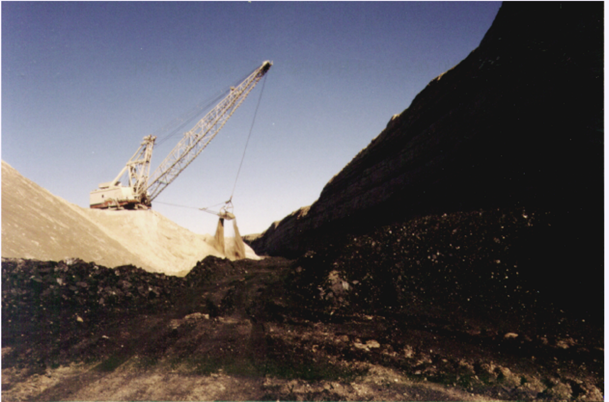
Figure MO-20. A Marion 8000-series dragline uncovering the Deadman coal bed.
