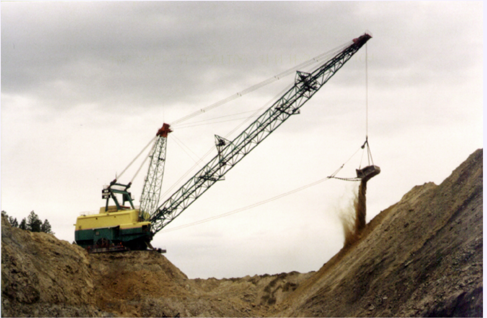
Figure MO-19. This Bucyrus-Erie 1570 dragline is sitting on the highwall side of the pit, moving overburden to the low wall or spoil side.
