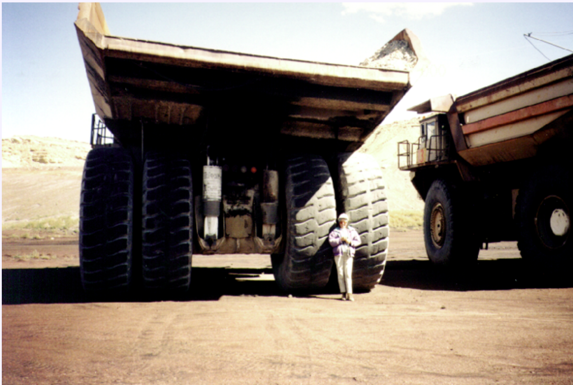
Figure MO-30. Large truck tires are an expensive part of haulage operations. These 10 ft diameter tires dwarf this geologist.
