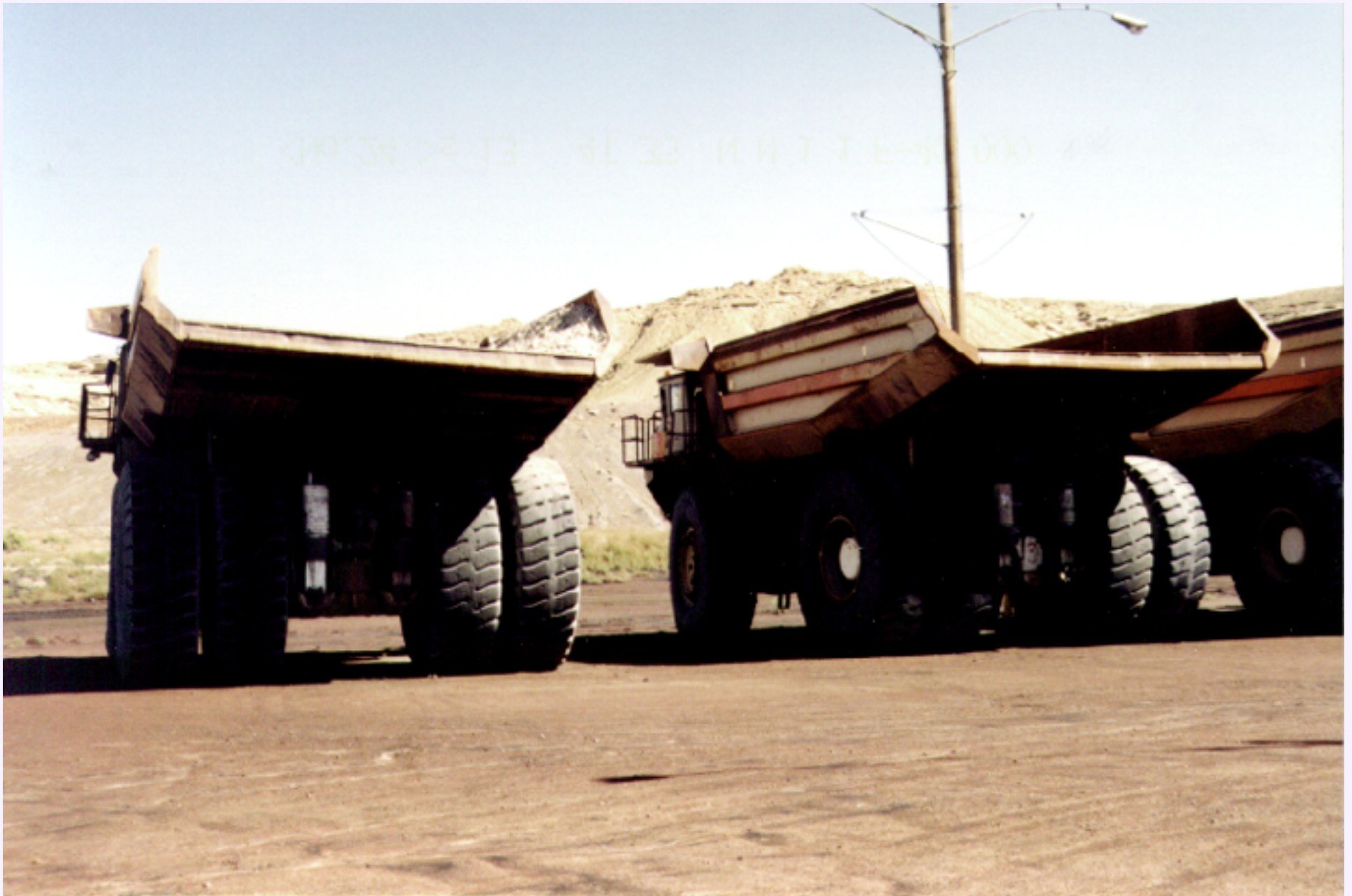
Figure MO-32. The ready line of spare trucks. Although end-dump trucks have high mechanical reliability, it is necessary to have enough spare equipment to maintain production when mechanical failures occur. Photograph by Ken Takahashi, 1999
