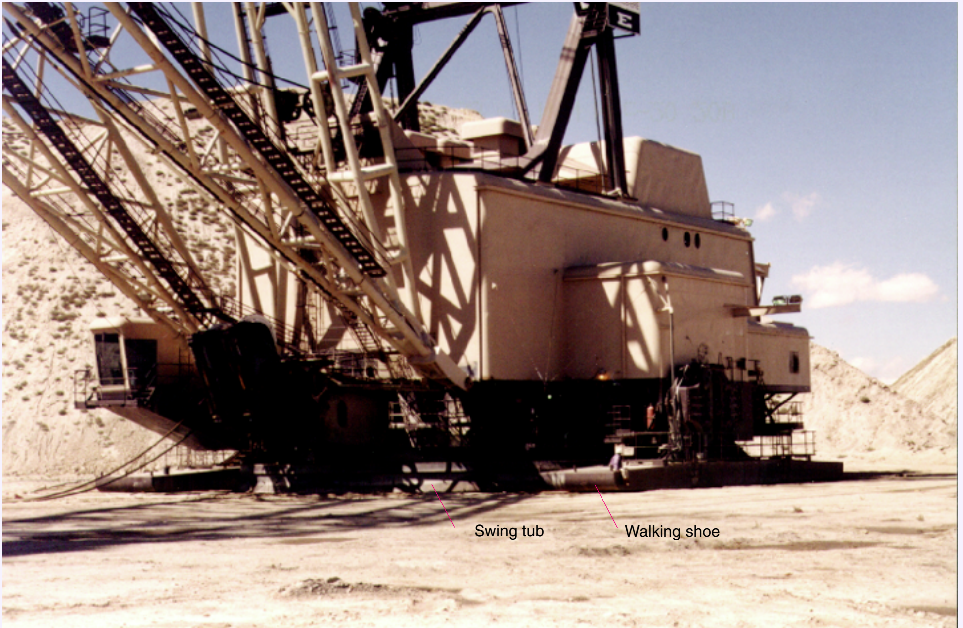
Figure MO-18. A Bucyrus-Erie 1570. Note the walking shoe used to move the dragline.
