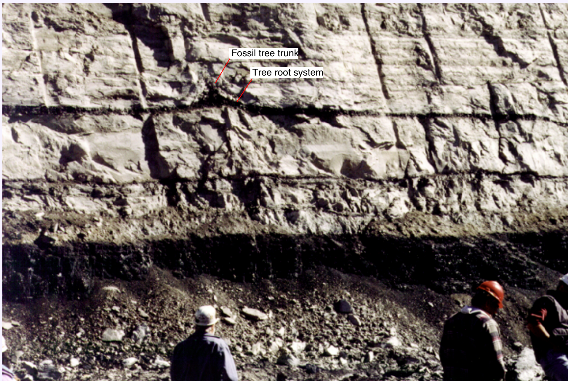
Figure MO-6. Highwall showing the Deadman coal bed in a dragline stripped pit. Note the fossilized tree trunk and root system in the thin coal bed in the overburden.
