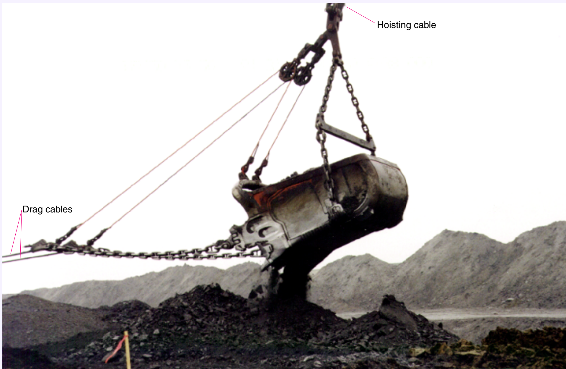
Figure MO-14. Digging and dumping operations of the dragline bucket are controlled by the hoist cables and the drag cables. (Note that this bucket is in a dumping position)
