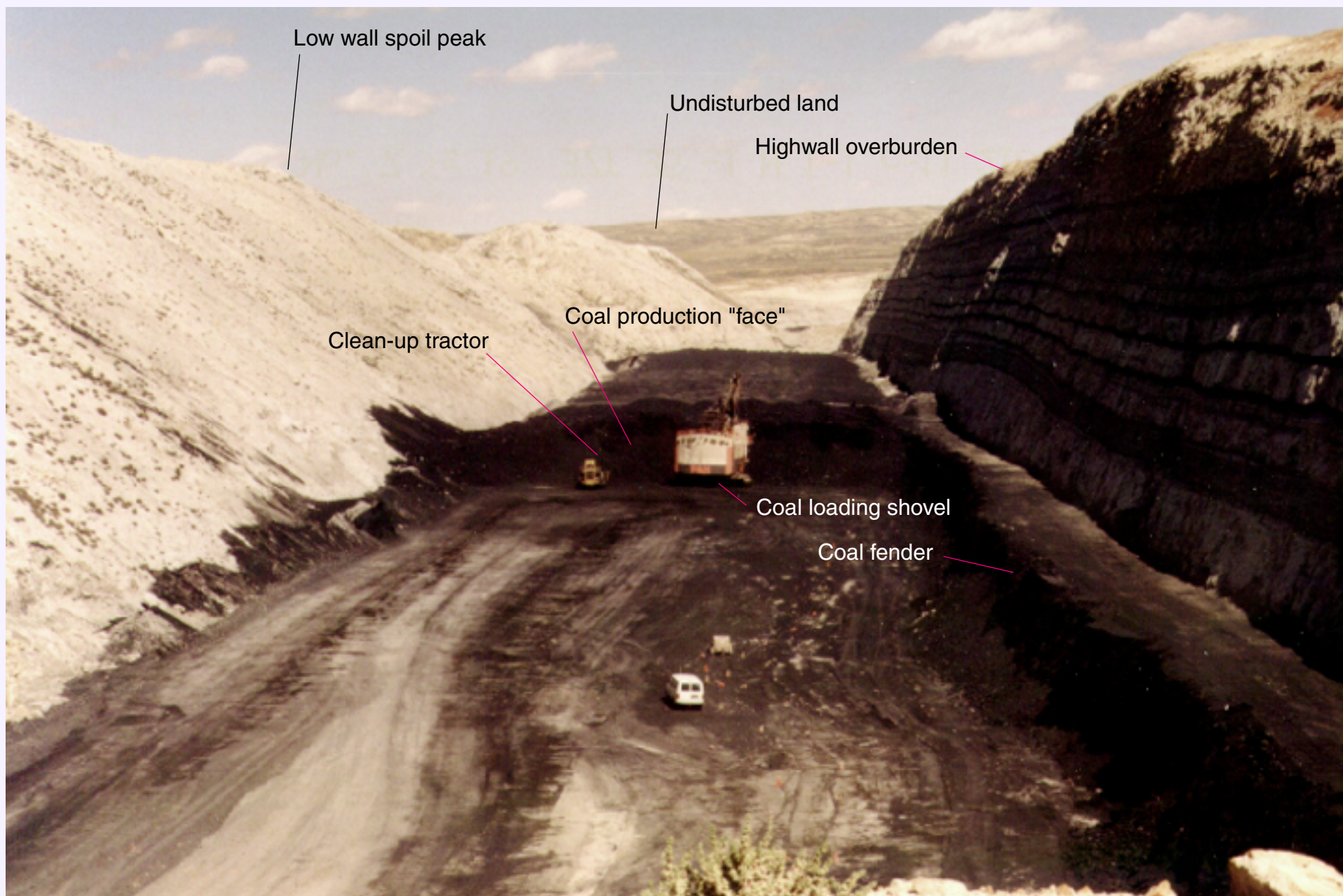
Figure MO-2. Coal removal from a dragline-stripped pit. Note the overburden spoils on the left, coal production "face" in the center, coal "fender" on the lower right and the highwall to the right.
