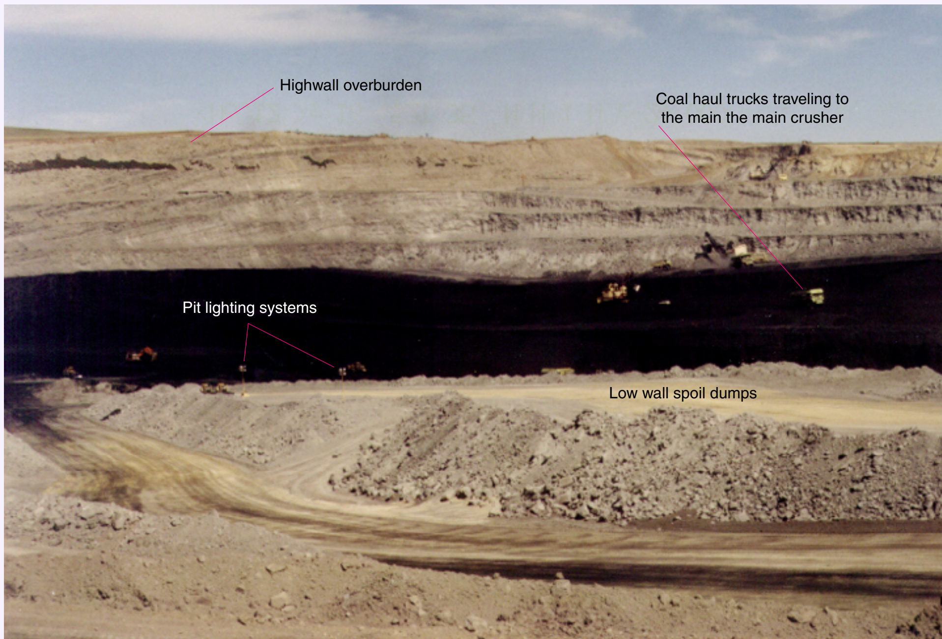
Figure MO-8. Truck-shovel stripping operations load and move overburden from the highwall side of the pit to low-wall dumps (foreground). The coal bed is removed and hauled to a primary crushing facility, thereby making more room for additional low wall spoil dumps.
