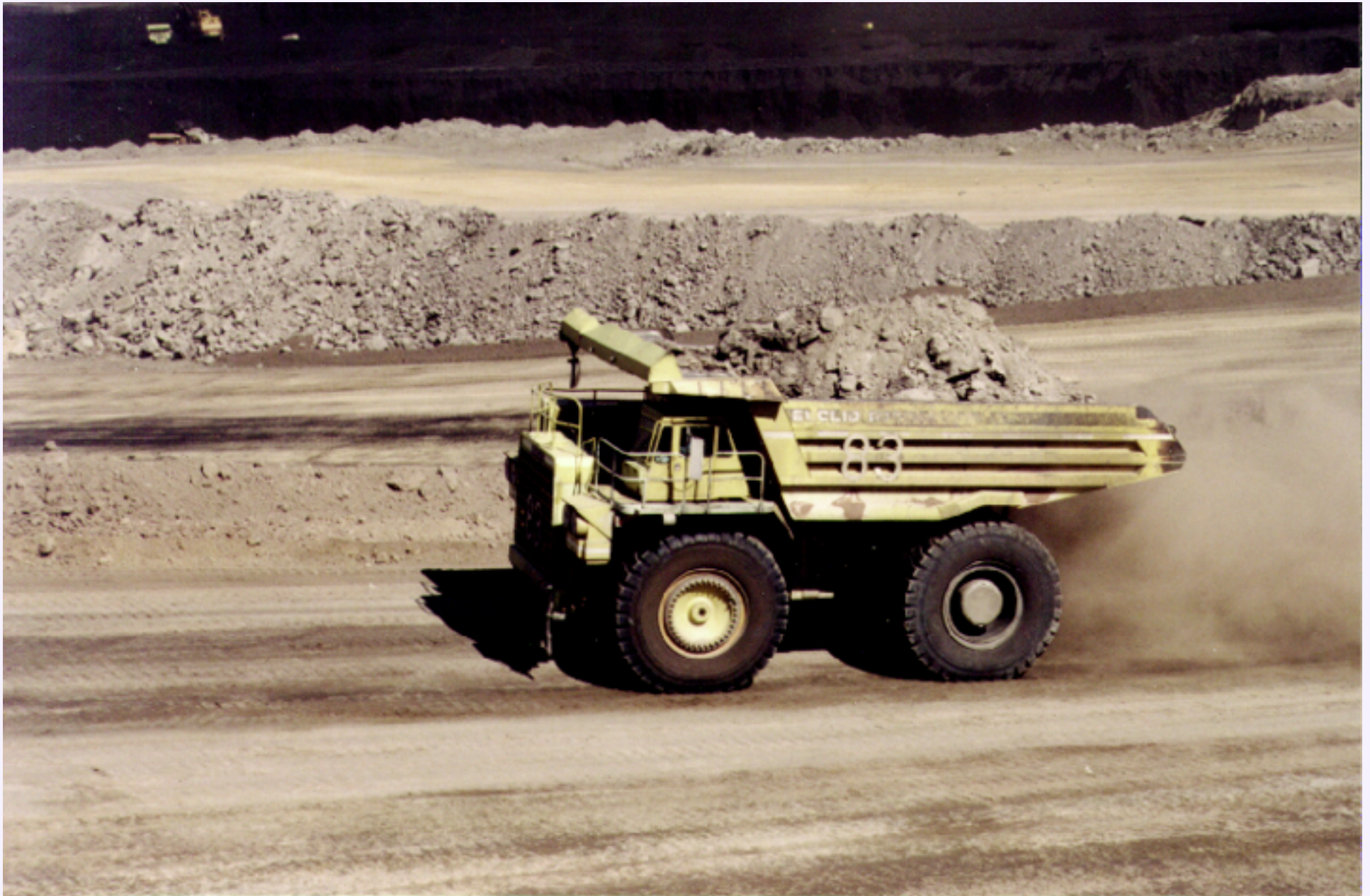
Figure MO-29. Depending on the size of the loading shovel, this Euclid end-dump truck can be loaded in 3-5 minutes.
