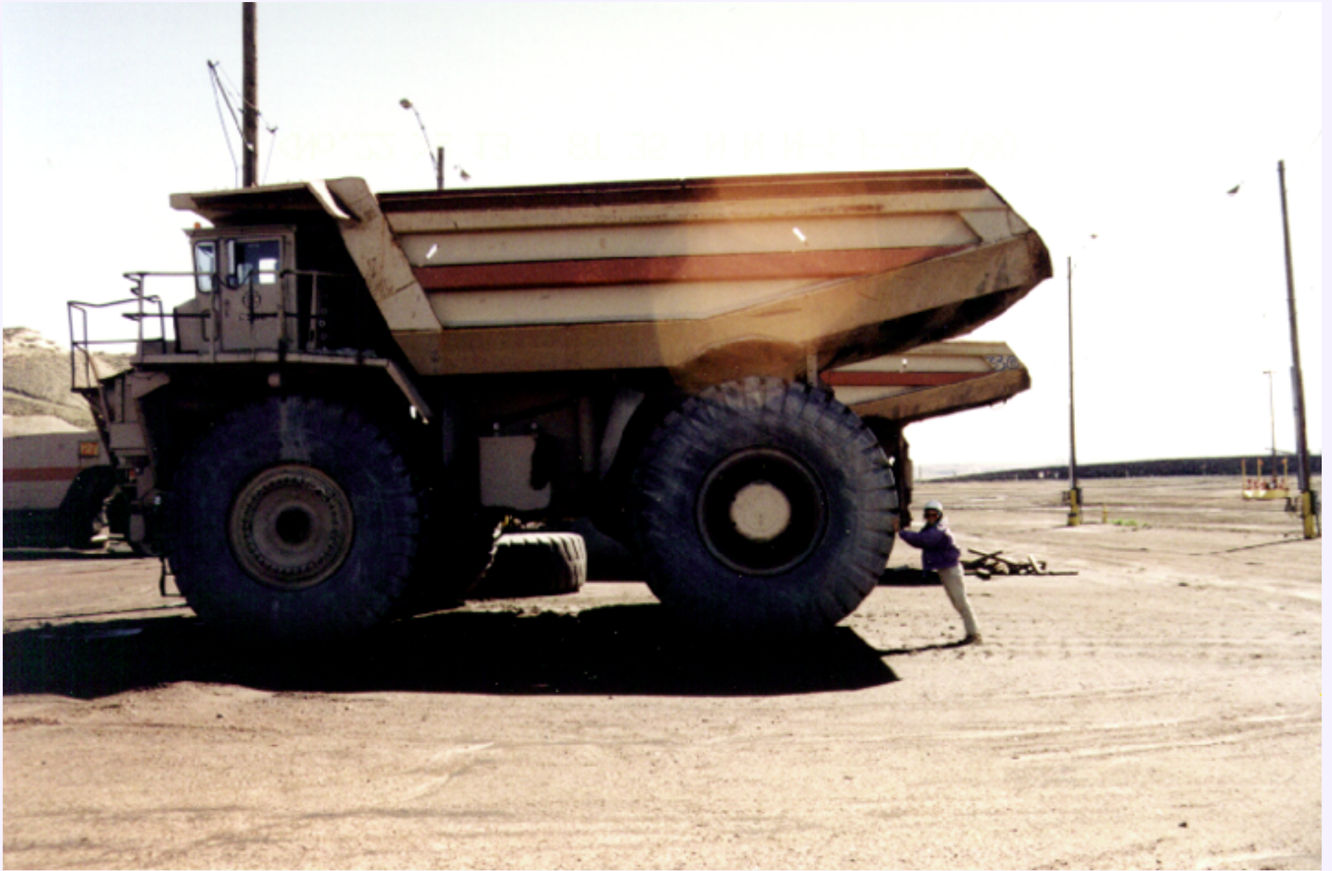
Figure MO-31. Large haul trucks can carry from 170 to 240 tons or more.
