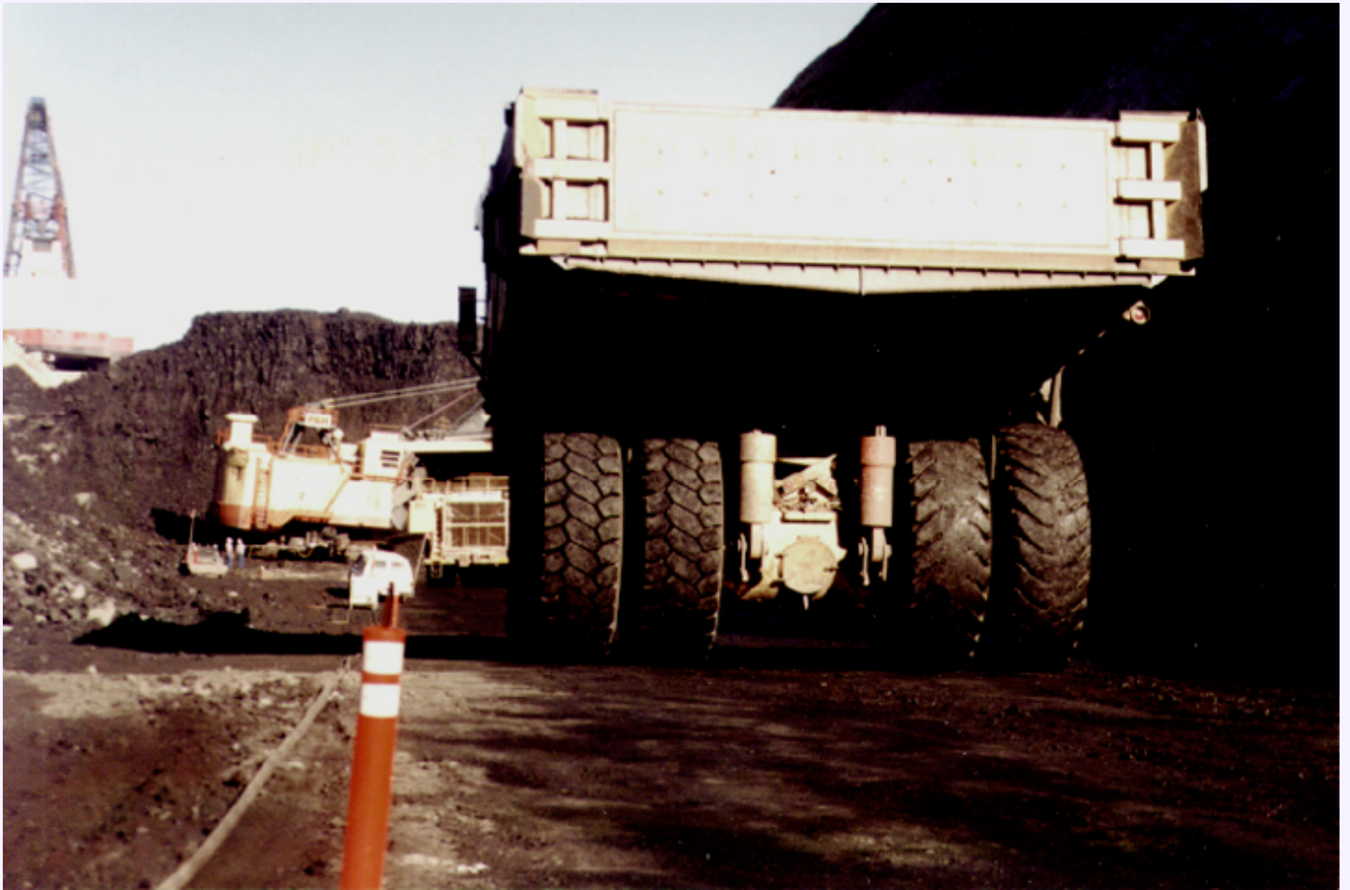
Figure MO-36. These Unit Rig end-dump trucks can carry as much as 240 tons of coal. These trucks are being loaded by a P&H shovel.
