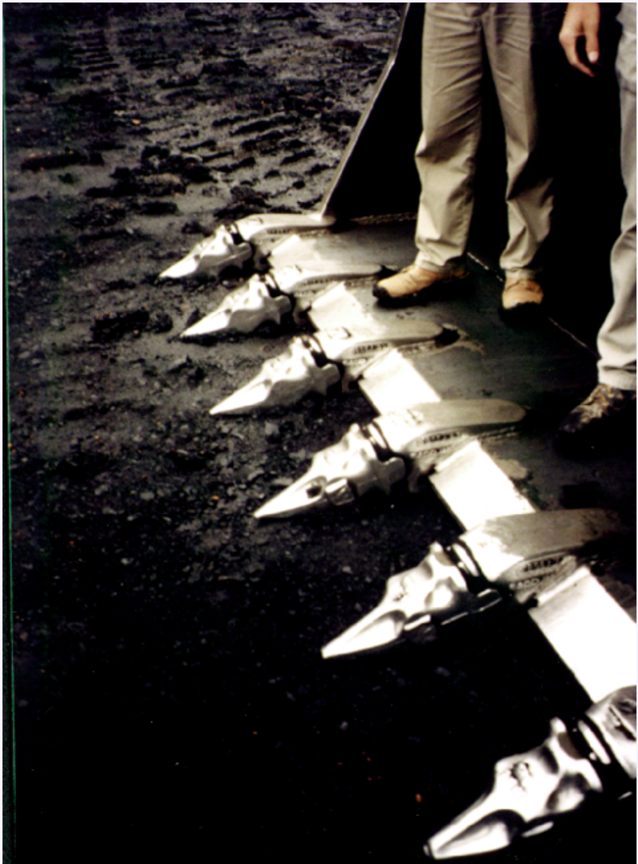
Figure MO-25. Front-end loader buckets used for loading coal vary in size depending on the strength of the coal, how well it is fragmented from blasting, and the production rates needed at the mine. This bucket is in the 15-20 cubic yard capacity class. Photograph by Ken Takahashi, 1999
