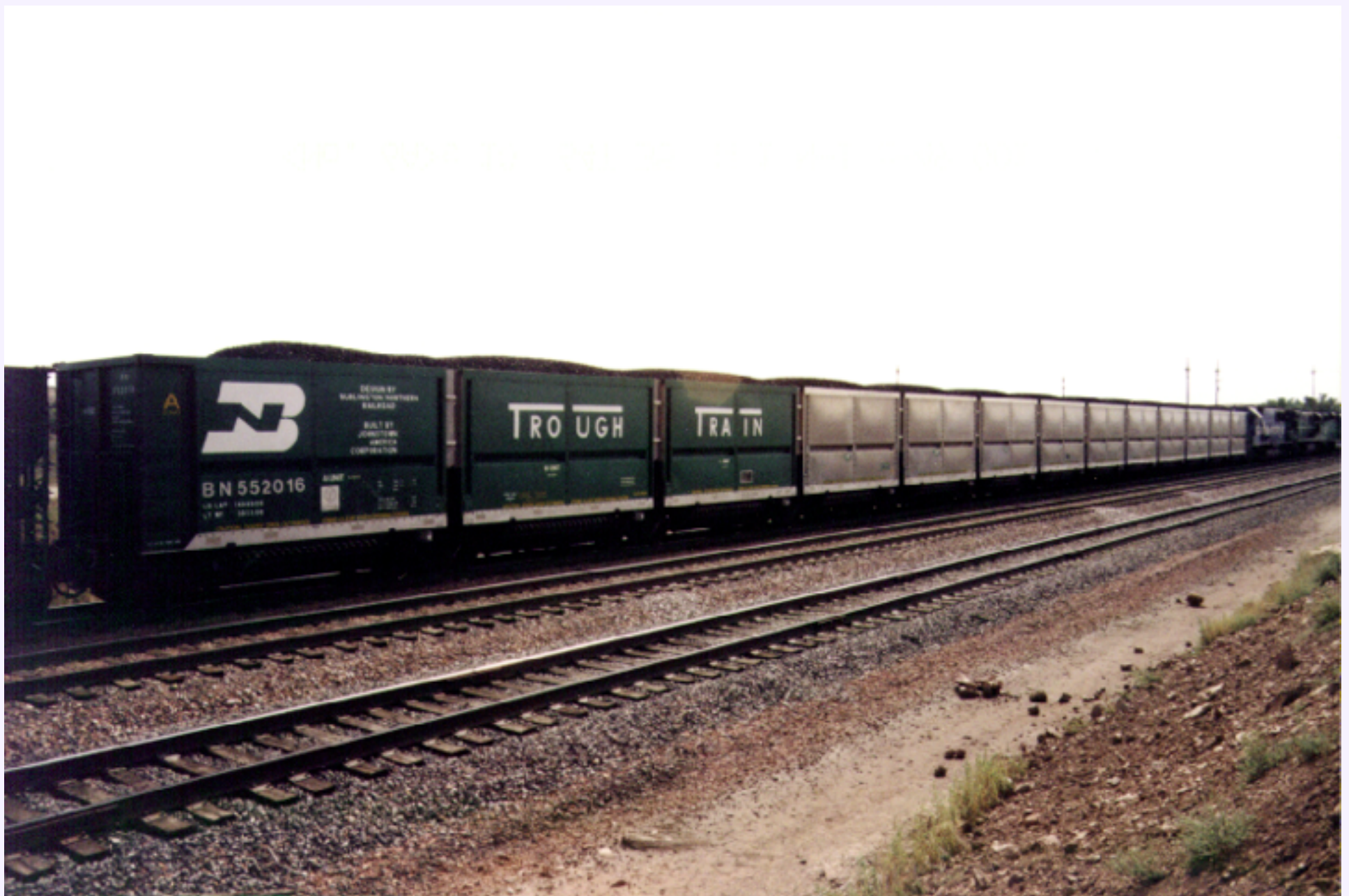
Figure MO-43. A trough train of normal length (one mile long) may carry as much as 50% more than a regular train with 100 cars, each carrying 100 tons.
