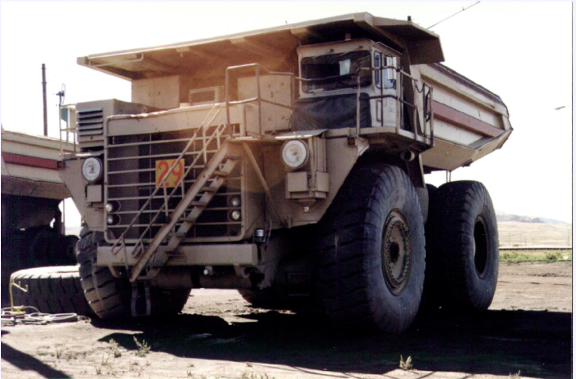
Figure MO-33. Cab access is in a high visibility location with guard rails and a large canopy to protect the operator from rock spillage during loading. Photograph by Ken Takahashi, 1999
