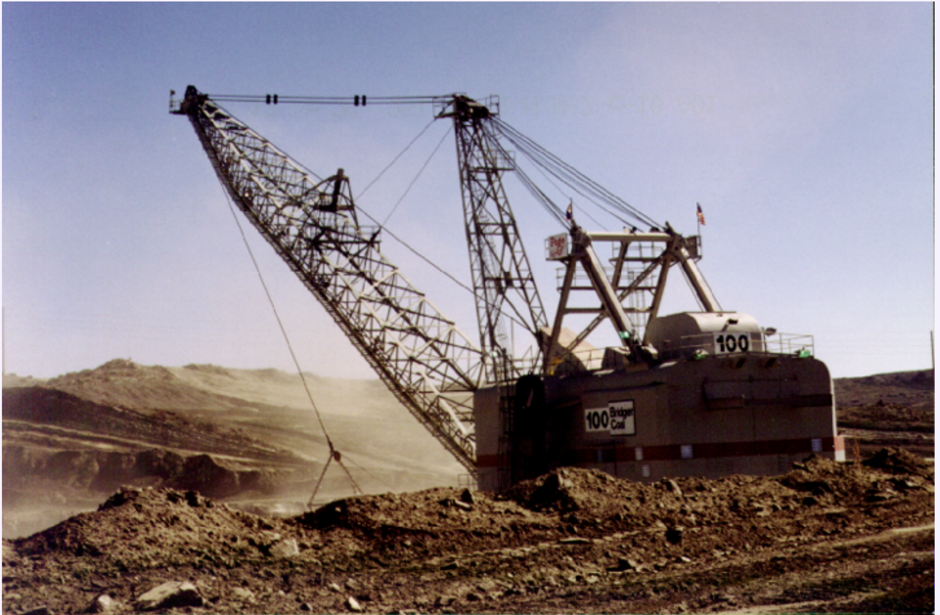
Figure MO-16. This Page dragline may be a Page 752 prototype. The Page 752 carries a 50-60 cubic-yard bucket.
