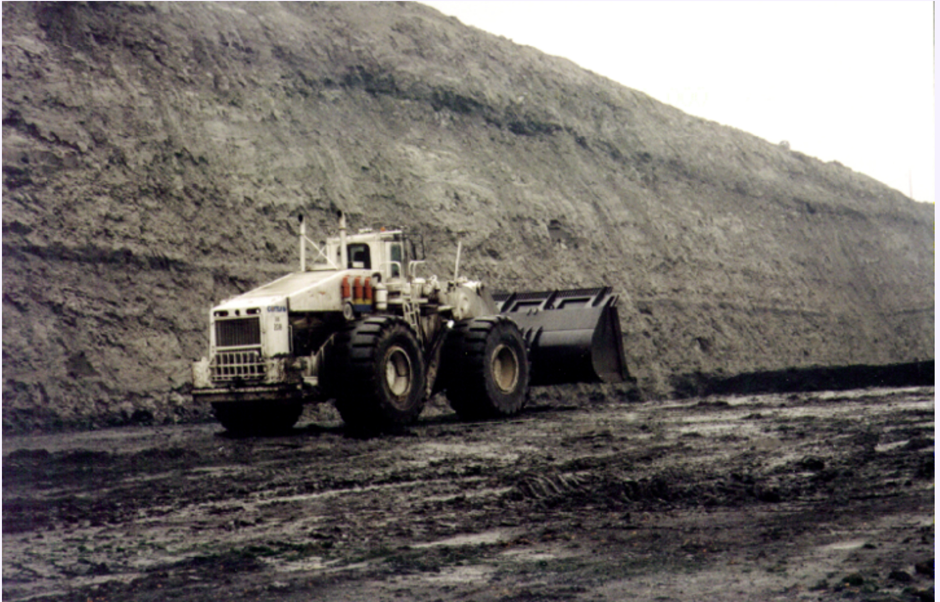
Figure MO-26. The ability to easily move from one location to another makes this Le Tourneau front-end loader a useful piece of production equipment.
