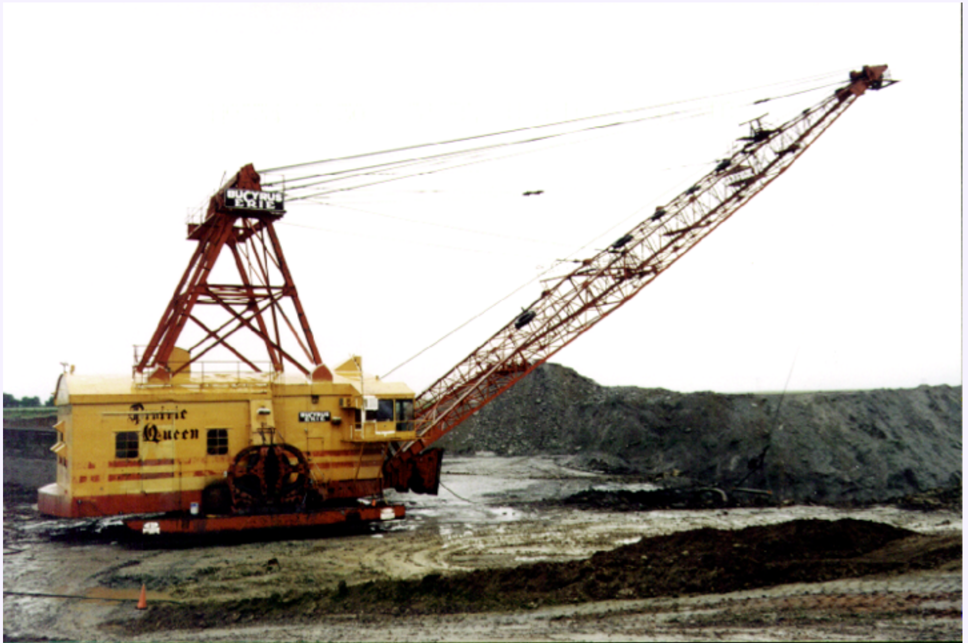
Figure MO-10. A medium-size Bucyrus-Erie dragline, nick-named "Prairie Queen" is stripping coal. Photograph by Ken Takahashi, 1999
