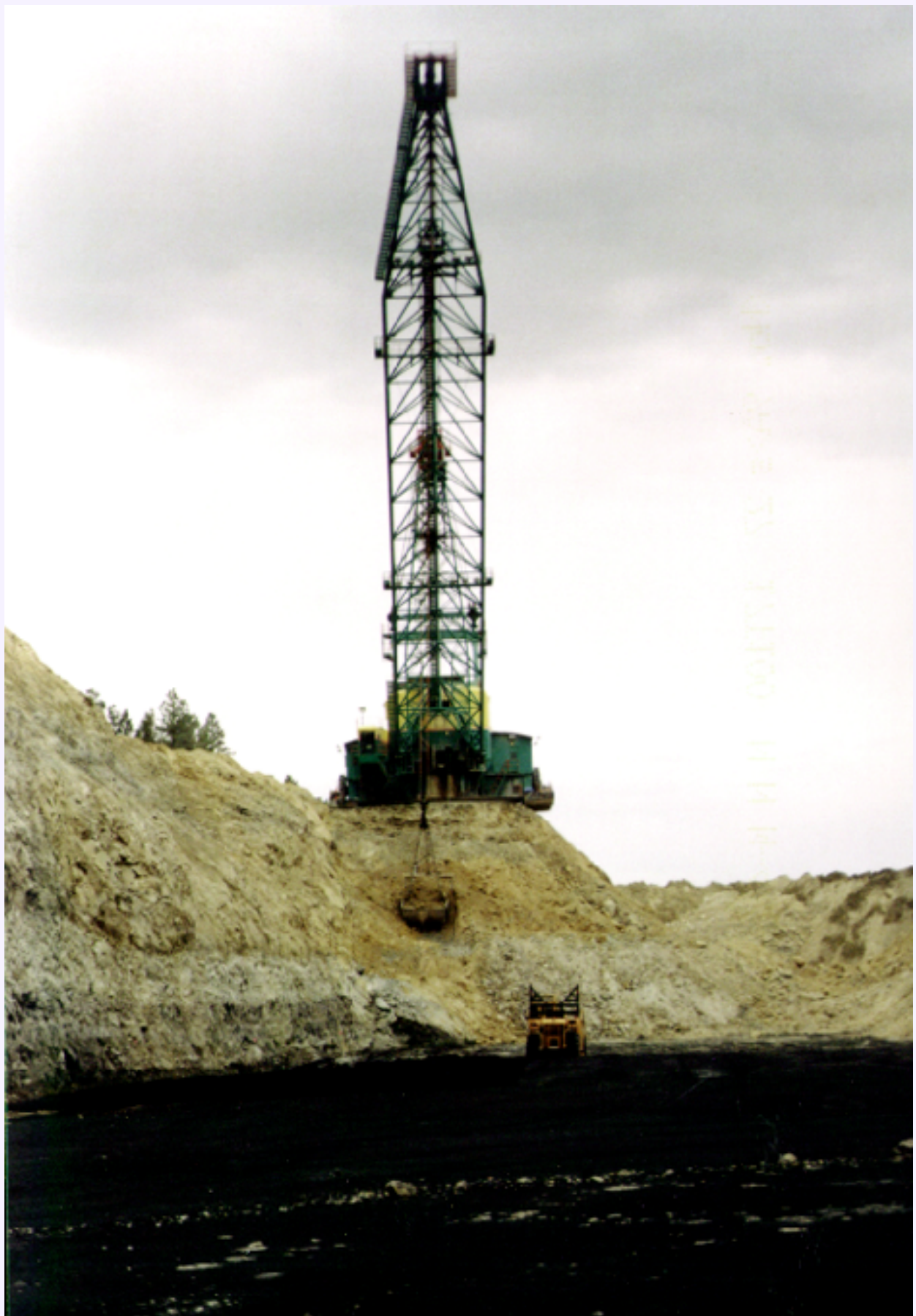
Figure MO-22. A Bucyrus-Erie 1570 dragline filling its bucket with overburden.
