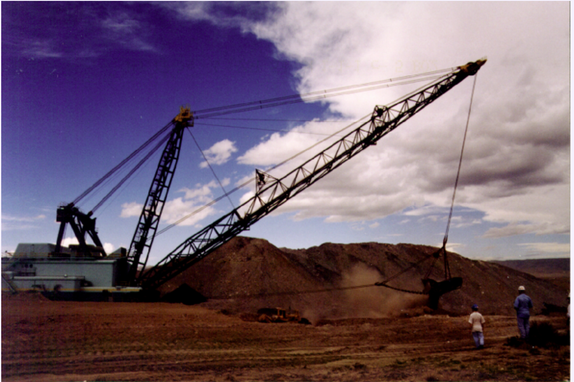
Figure MO-11. This Bucyrus-Erie 1570 dragline has a 72 cubic-yard bucket capacity and a 320 ft boom. Photograph by Ken Takahashi, 1999
