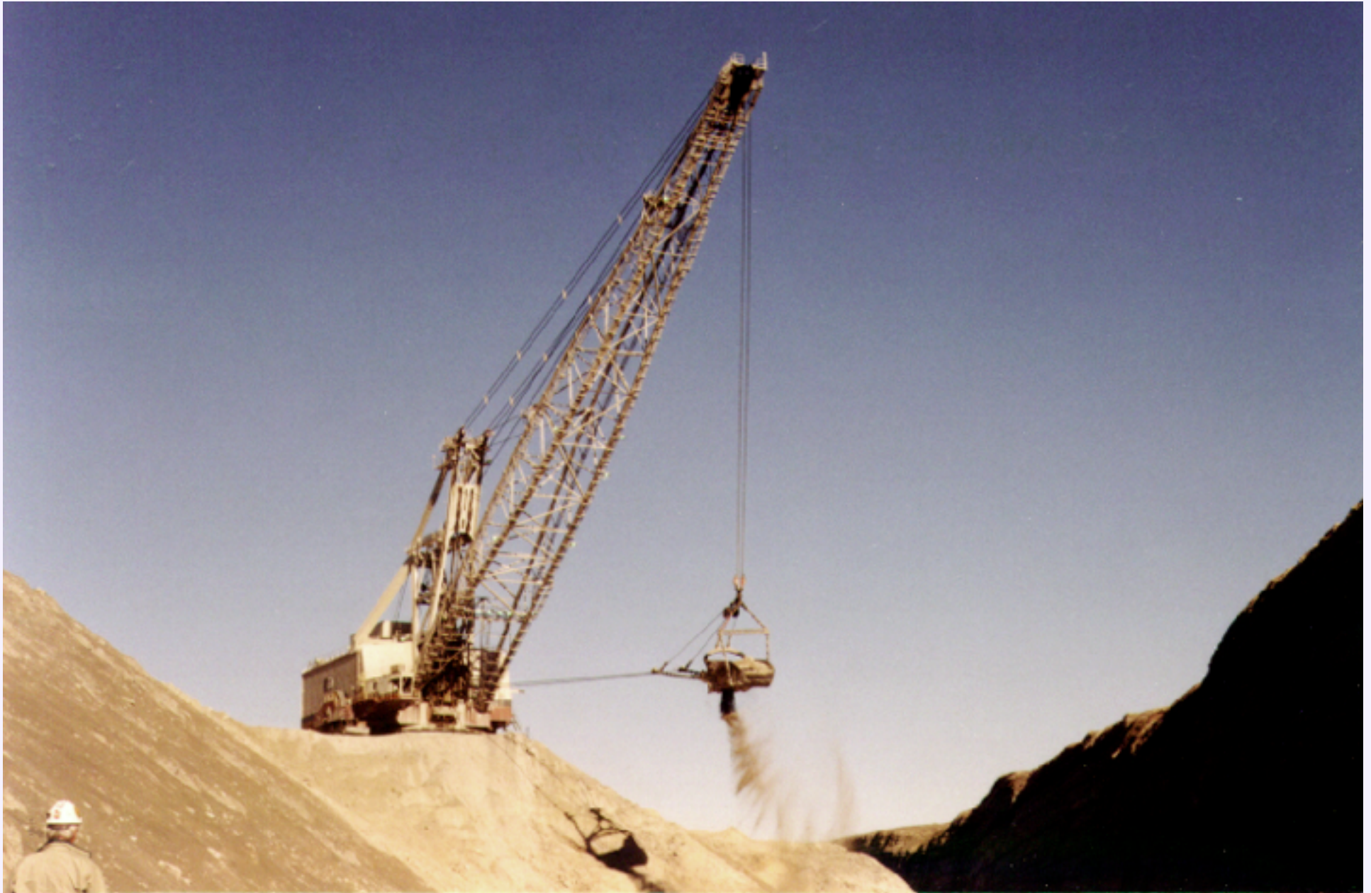
Figure MO-17. This Marion 8000-series dragline is working from an extended low wall bench.
