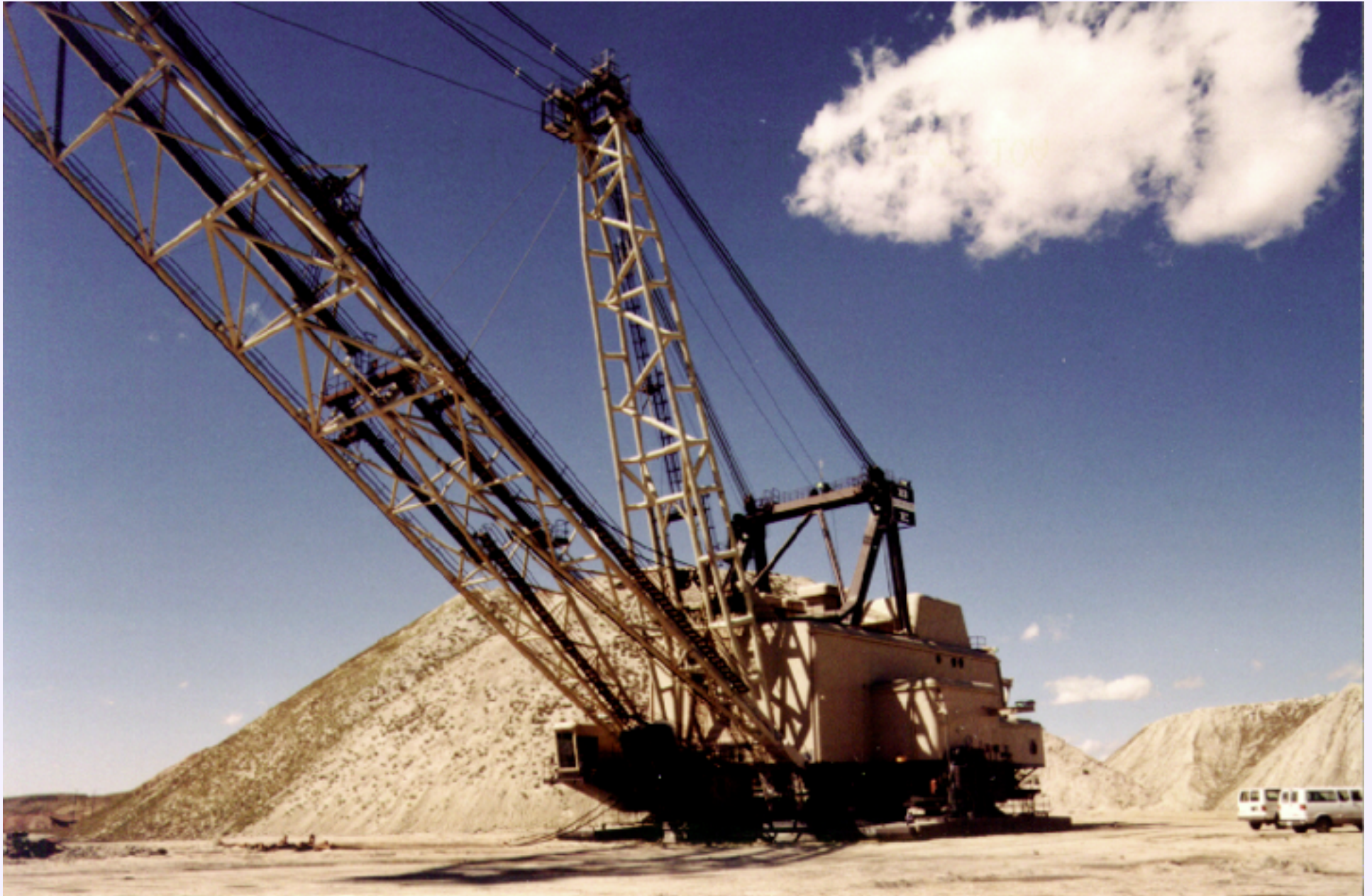
Figure MO-15. The Bucyrus-Erie 1570 is a larger size dragline. Each machine is designed for specific operating conditions. As the boom is lengthened, the cable drums inside the "house" must be increased in size to provide storage of the additional cable. Likewise, the bucket may be downsized to allow for additional boom length.
