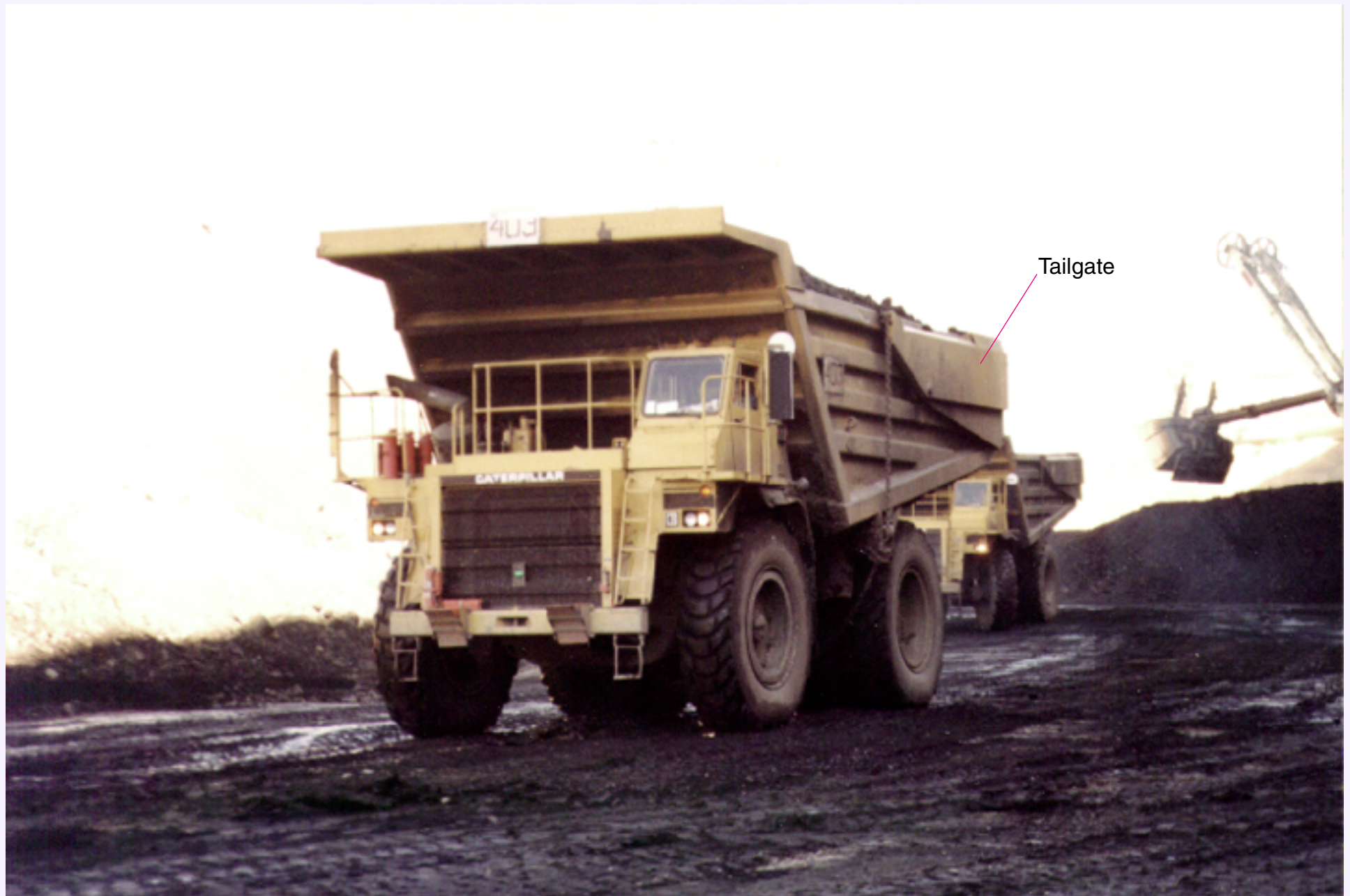
Figure MO-35. This Caterpillar 785 end-dump truck is hauling approximately 150 tons of coal to a primary crusher. The tailgate may increase the truck's capacity by 7 to 10%.
