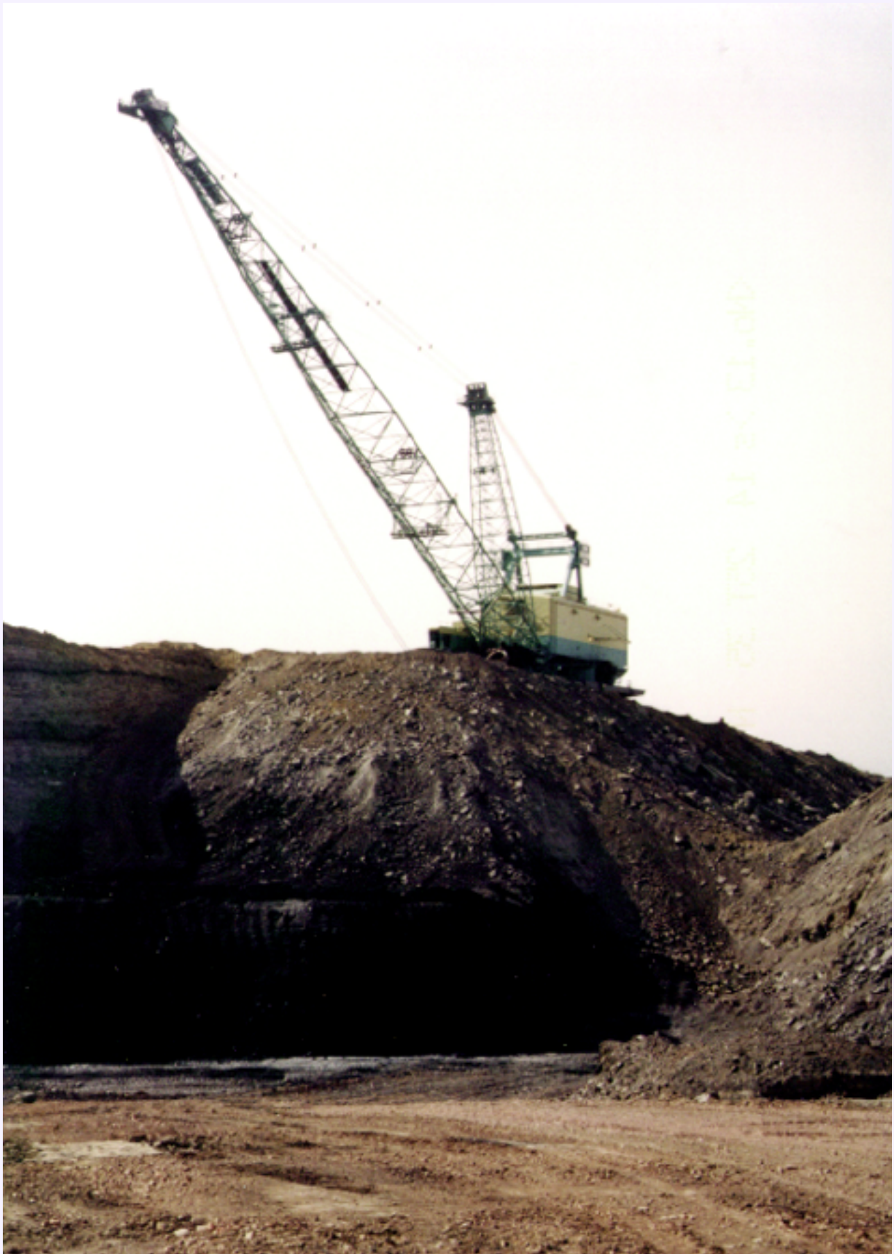
Figure MO-21. Standing on the pit access road looking at a thick coal bed and a Bucyrus-Erie 1570 dragline on the highwall side of the pit. Photograph by Ken Takahashi, 1999
