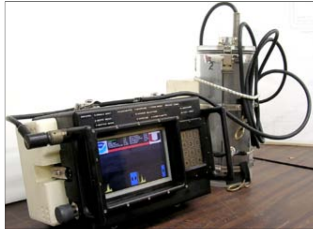
Figure 1. The diver-held stereo video camera showing the display screen and the control keypad.
