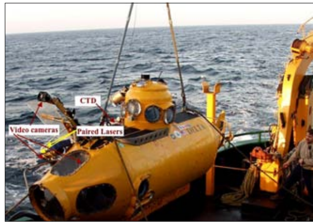
Figure 1. The Delta research submersible accommodates one scientific observer and one pilot, has a maximum operating depth of about 350 m, and a cruise speed of 1.5 knots. We equipped the submersible with three video cameras: a low-light, wide-angle black-and-white CCD camera positioned externally on the bow; a High-8 color video camera and associated lights externally positioned on the starboard side and flanked by paired lasers at a distance of 20 cm apart; and a hand-held digital video camera positioned inside the submersible in the lower port on the starboard side. (photo credit: M. Yoklavich)
