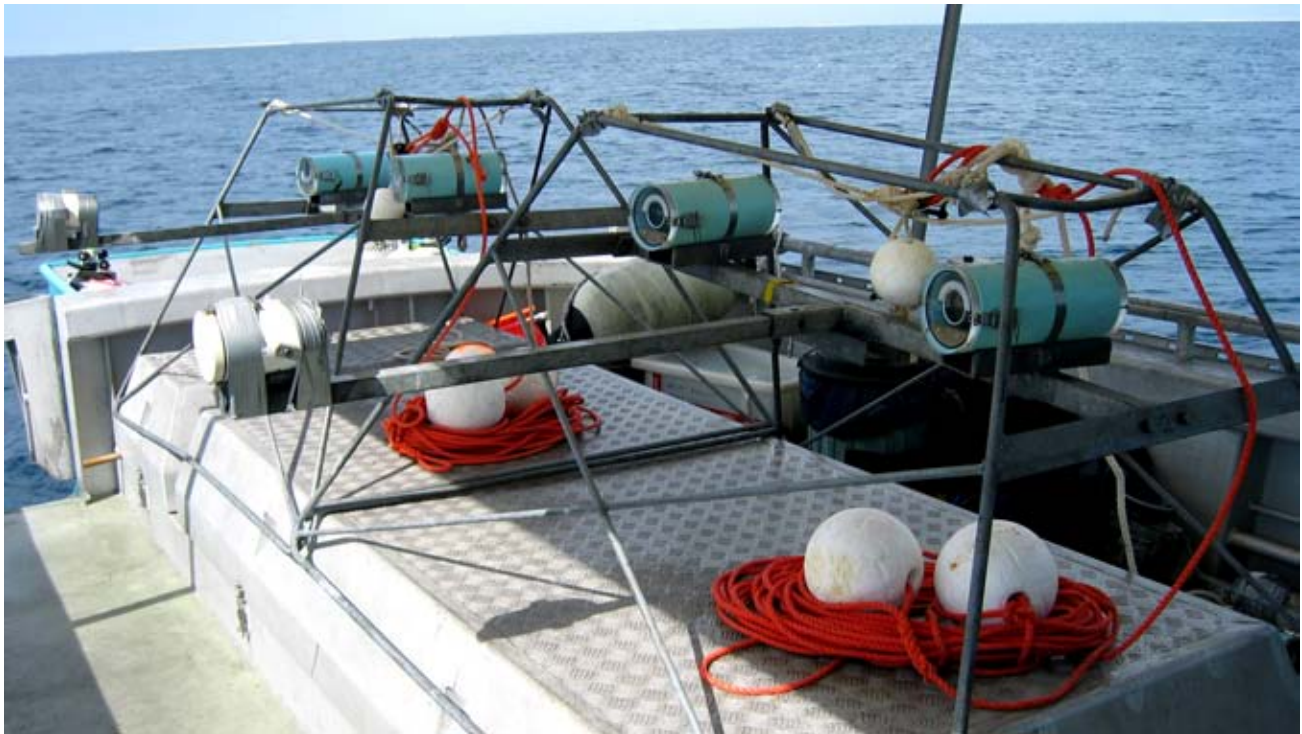
Figure 2. Two stereo BRUVS ready for deployment. These systems use off-the-shelf single CCD Sony HandiCams in PVC housings with acrylic ports.
