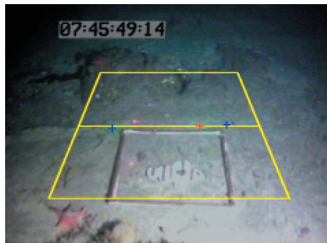
Figure 2. A view of the bottom with the quadrature superimposed. Note the square meter target on the bottom and the three reference laser points (red dots).
