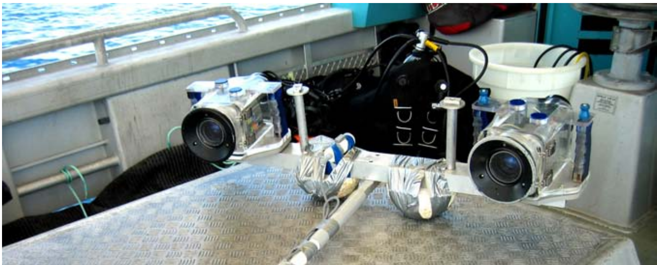
Figure 1. A diver-held stereo-video camera system. A SCUBA diver swims the camera system recording observations and comments directly onto one of the videotapes using a full-face mask containing a microphone (right).
