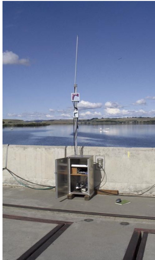
Figure 2. The wireless arrangement for one receiver-antenna combination (not shown) installed on the deck of the McNary Dam. All of the receivers are connected to a local computer, which can be accessed through the Internet.
