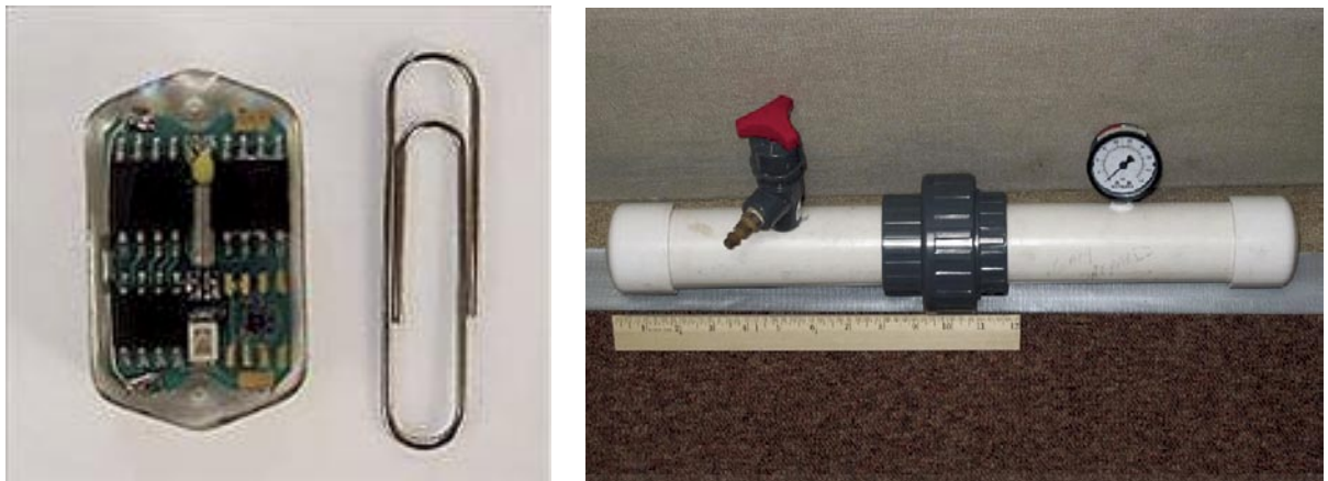
Figure 1. Lotek 1100 data storage tag (left, shown to scale against a paper clip) and a pressure chamber used for predeployment testing (right, shown to scale against a ruler).
