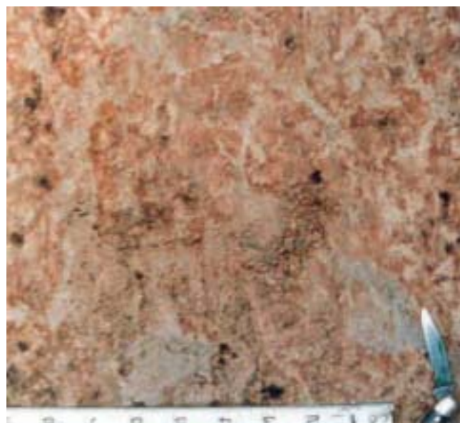
Figure 31. Indicator F12 Iron/Manganese Masses in a 40 percent depleted matrix. Scale is inches.
