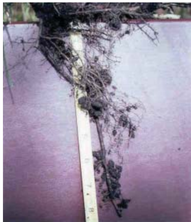
Figure 11. Indicator A6 Organic Bodies. The organic bodies are approximately 1 to 3 cm in diameter; sometimes they are smaller. Scale is inches.
