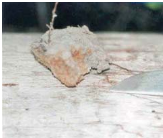
Figure 38. Redoximorphic features as required in many of the Indicators. These redox concentrations occur as pore linings along root channels and ped faces.
