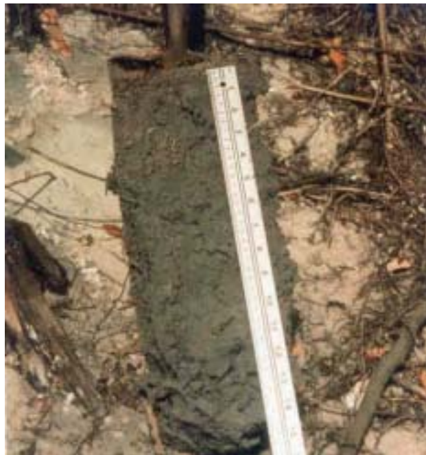
Figure 14. Indicator S4 Sandy Gleyed Matrix. The gleyed matrix begins at the soil surface. Scale is inches (R) and cm (L).
