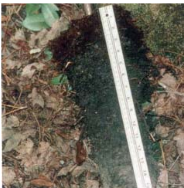
Figure 13. Indicators A8 Muck Presence and S7 Dark Surface. Muck is less than 1 cm thick and the dark surface is 18 cm thick. Scale is inches (R) and cm (L).
