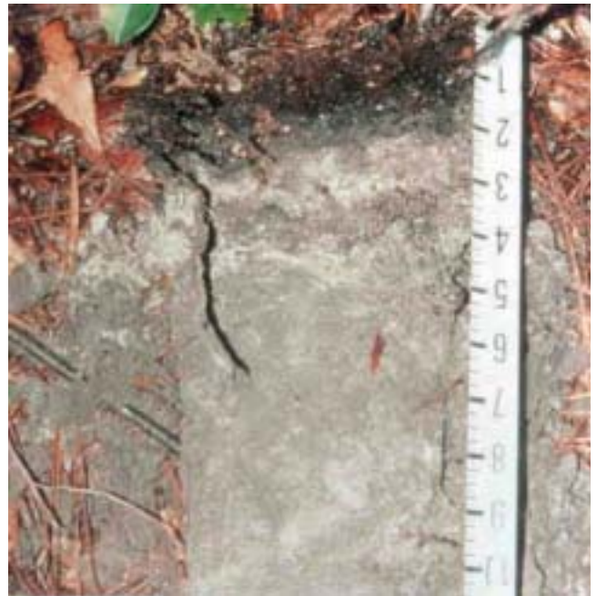
Figure 17. Indicator S6 Stripped Matrix. The matrix stripped of organic matter begins beneath the surface layer. Scale is inches.
