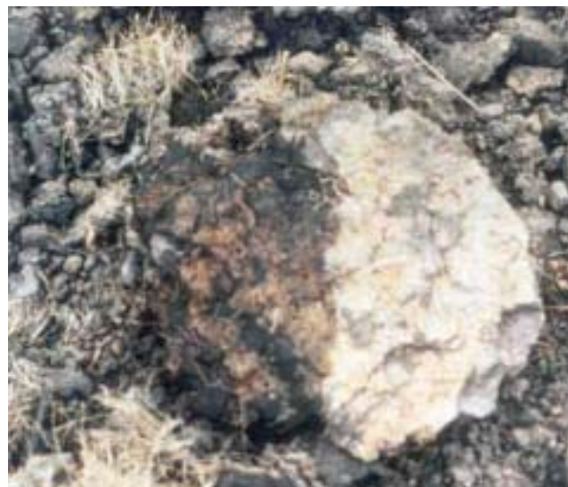
Figure 3. Indicator F6 Redox Dark Surface. The left is moist and the right is dry. Most commonly moist soil colors are to be used when identifying and delineating hydric soils.
