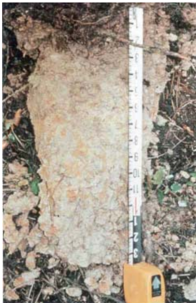
Figure 23. Indicator F3 Depleted Matrix. The chroma is 2 below a depth of about 15 cm. Redox concentrations are present. Scale is inches.
