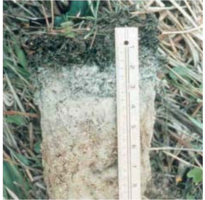
Figure 16. Indicator S6 Stripped Matrix. The matrix stripped of iron oxides begins below a depth of about 10 cm. Scale is inches (R) and cm (L).
