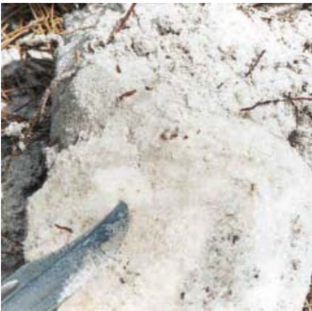
Figure 18. Indicator S6 Stripped Matrix. Close up of oval stripped areas showing the associated decomposing roots.
