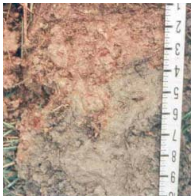
Figure 24. Indicator F3 Depleted Matrix. The chroma is 1 within a depth of about 10 to 15 cm. Redox concentrations are absent. Scale is inches.
