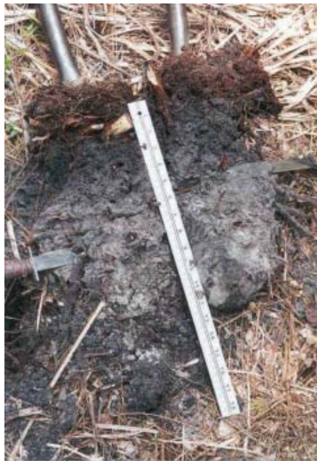
Figure 1. The field indicators are to be used to delineate hydric soils. The soil on the right is hydric that has the Indicator S6 Stripped Matrix starting at a depth of about 14 cm, and the soil on the left is nonhydric with the Stripped Matrix starting at a depth of about 18 cm.
