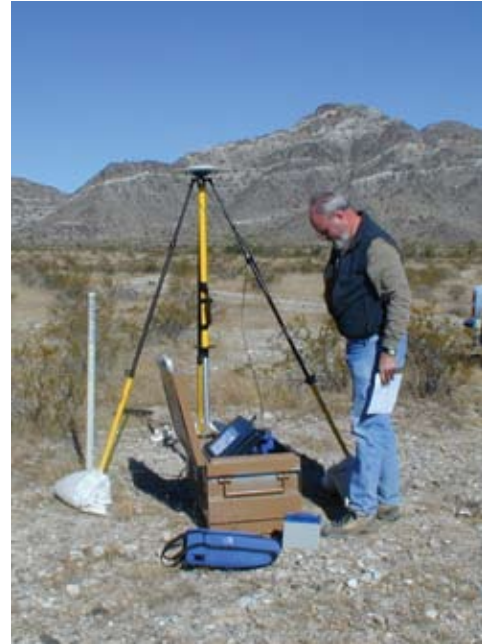
Figure 8.4. Since 2002, NOAA has made available to the public OPUS, the Online Positioning User Service. This tool, the culmination of years of GPS research and CORS infrastructure building, allows anyone with a single geodetic-quality GPS receiver to position themselves in the National Spatial Reference System to an accuracy of two centimeters with just two hours of data. Further research is ongoing to reduce the amount of field time to just minutes. The number of users has grown from about 1,000 per month in FY2002 to over 13,000 per month in FY2005.
