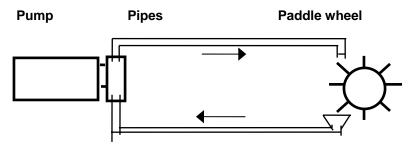
So, in a circuit, the electrons are always there. All a generator does is get the electrons moving down the wire (flow of electricity). The energy of their movement is what powers the light bulb, just like the flow of water is what turns the paddlewheel. No electrons get "used" up; instead they are returned to the generator by the second wire.
