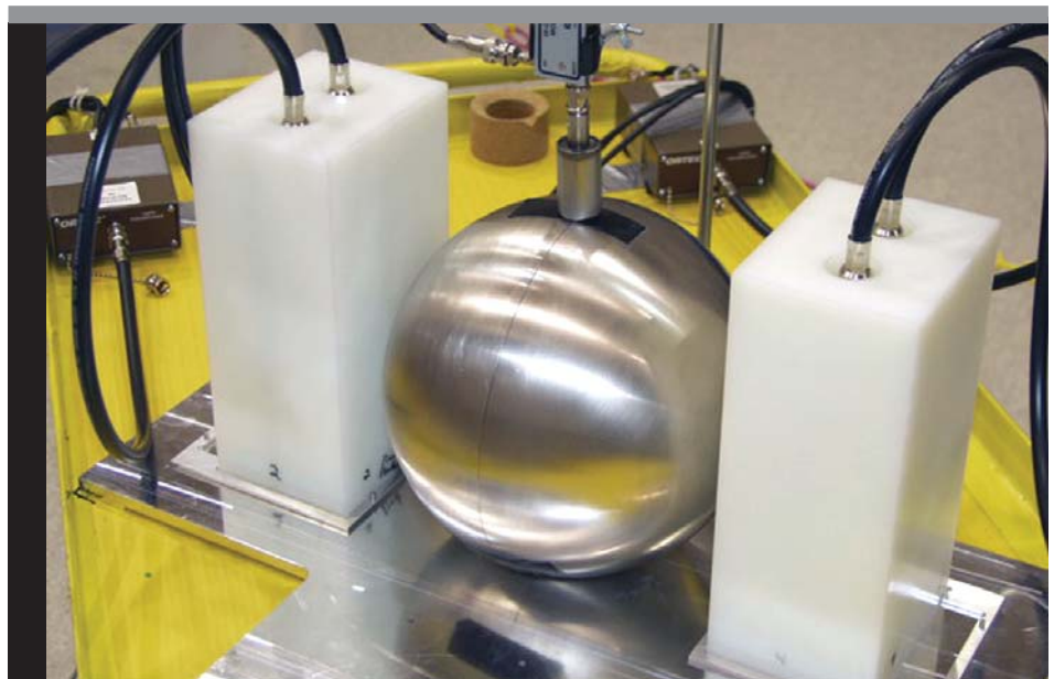
CRITICALITY SAFETY: NNSA's Device Assembly Facility at the Nevada Test Site (NTS) is home to experiments like this one, a test of how well nickel acts as a neutron reflector. Pictured is a 4.5 kg ball of alpha-phase plutonium surrounded by three inches of nickel nesting shells. Data from the Energy Nuclear Criticality Safety Program test will be used to develop criticality safety benchmarks. See pages 4 and 5 for more on the diverse activities at NTS.
