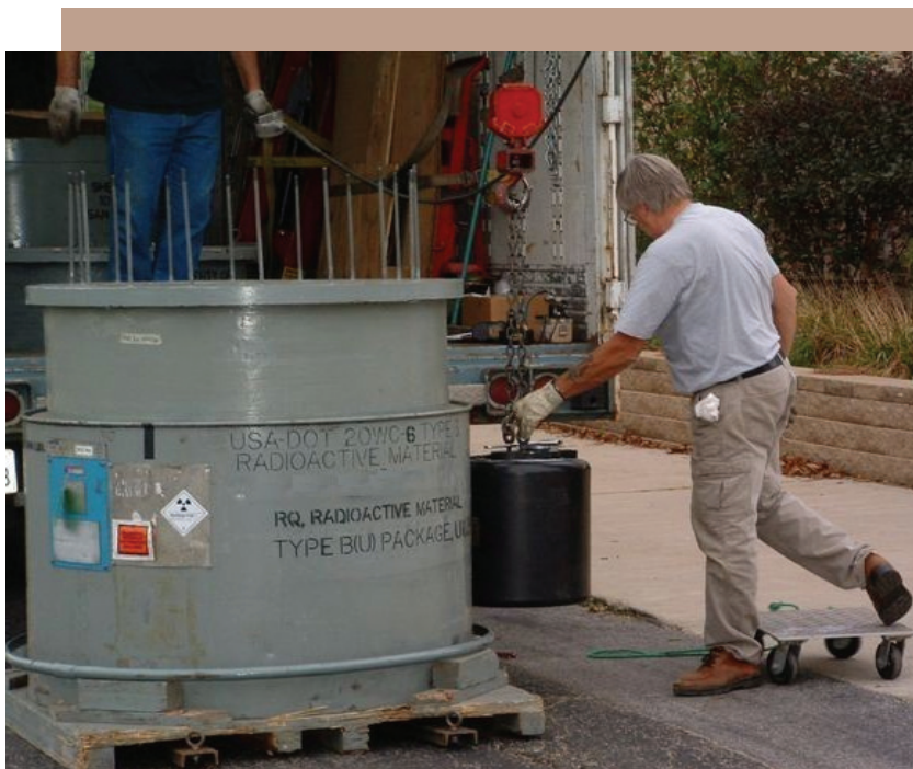
RADIOACTIVE SOURCE RECOVERY: OSRP contractors hoist a Cesium-137 irradiator into a Type B shipping container at an Illinois high school.
