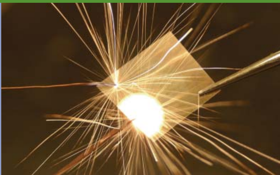
NANOFOIL: Reactive NanoTechnologies' NanoFoil is a nanoengineered heat source developed with Lawrence Livermore National Laboratory and Johns Hopkins University. An electrical pulse applied to the foil initiates a chemical reaction to produce high temperatures. The invention won an R&D 100 Award for 2004. See page 5 for a description of all the R&D 100 awards won by NNSA laboratories.
