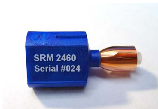
SRM 2460 mounted on a blue stub
