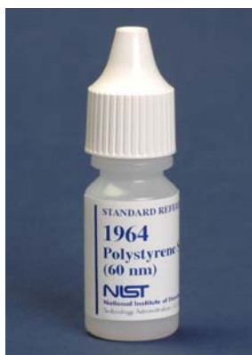
Nominal 60 nm Diameter Polystyrene Spheres
