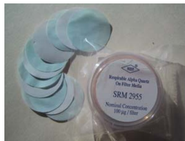
The loaded PVC filters and blue spacers in SRM 2955.
