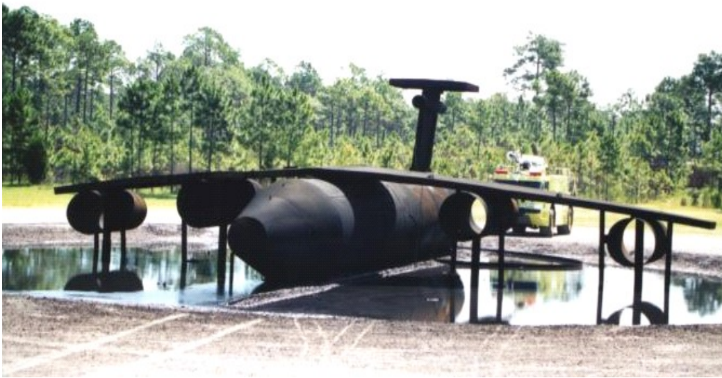
Figure 7. Large-Scale, 100-ft-Diameter Fire Burn Area With Aircraft Mockup
