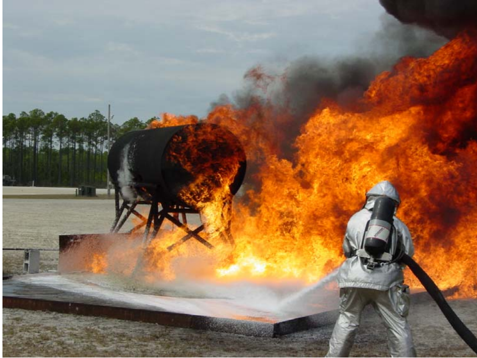
Figure 12. Fire Fighter Extinguishing F-100 Engine Nacelle With Concrete pad
