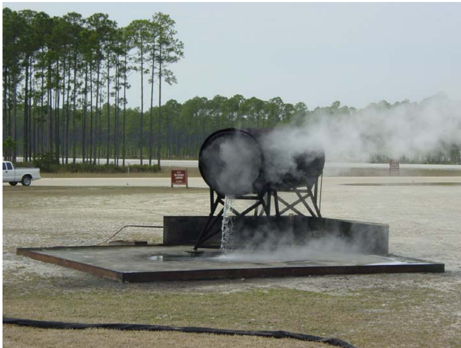
Figure 6. F-100 Engine Nacelle With Concrete pad
