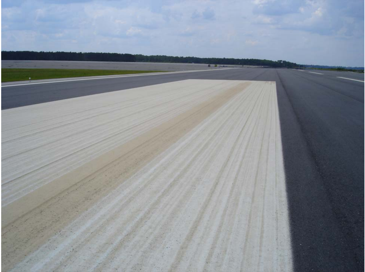
FIGURE 3. WHITE PAINT MARKINGS WITH ADSIL AND TYPE I BEADS
