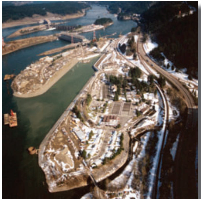
Tower, gates and navigation lock nearing completion. Earth removal opened the downstream to the Columbia River.
