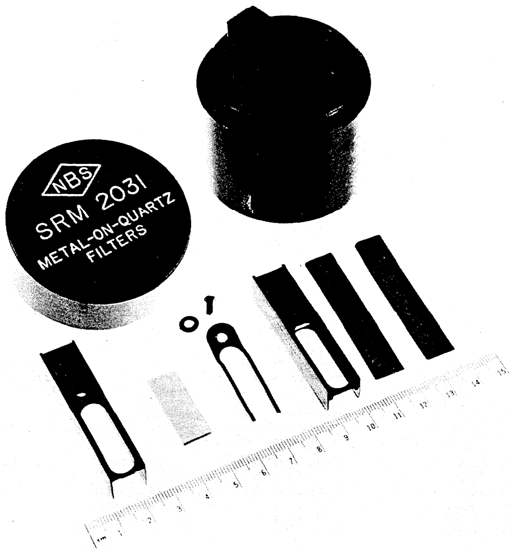
Figure 16. Illustration of SRM 2031, Metal-on-Quartz Filters for Spectrophotometry. This same figure illustrates the certificate for SRM 2031. See text for details.
