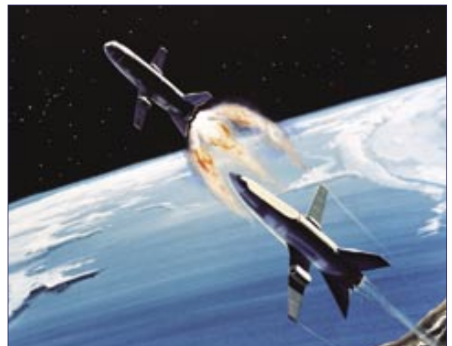
Figure 1.1-1. Early concepts for the Space Shuttle envisioned a reusable two-stage vehicle with the reliability and versatility of a commercial airliner.
