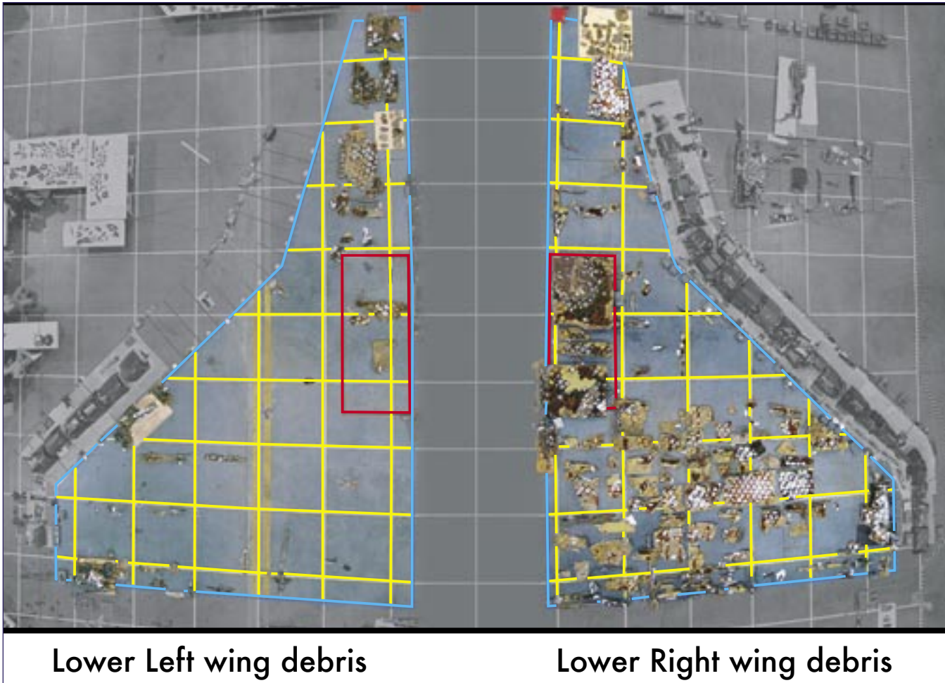
Figure 3.7-1. Comparison of amount of debris recovered from the left and right wings of Columbia. Note the amount of debris recovered from areas in front of the wheel well (the red boxes on each wing) were similar, but there were dramatic differences in the amount of debris recovered aft of each wheel well.
