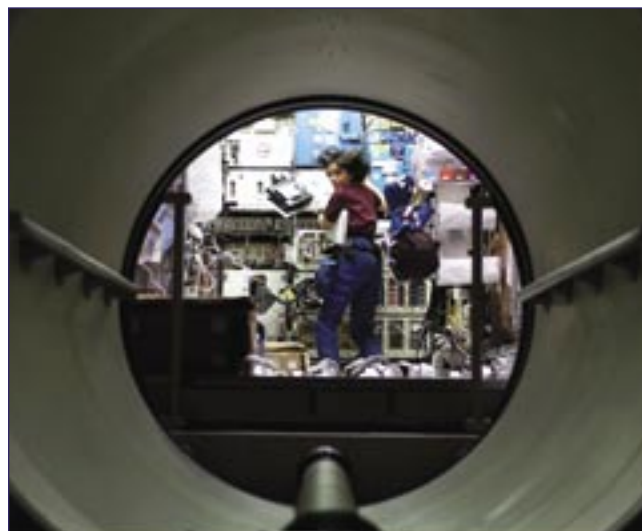
Figure 2.4-1. The tunnel linking the SPACEHAB module to the Columbia crew compartment provides a view of Kalpana Chawla working in SPACEHAB.
