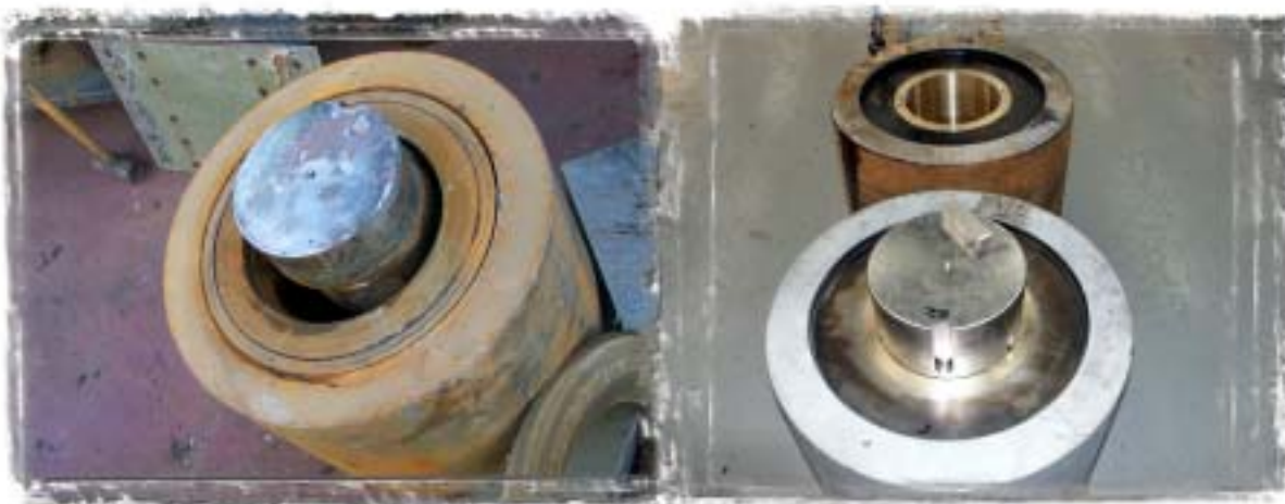
Left -- the old bushing and roller are displayed prior to its replacement. Right -- the new bushing and roller are displayed.
