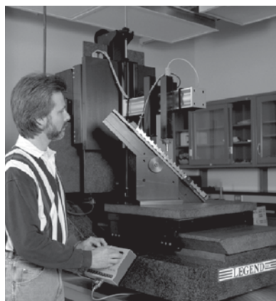
The Electronic Measuring Device's Legend coordinate measuring machine
