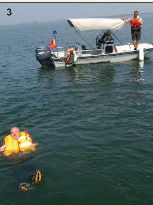
Nathan Dinehart, a park ranger at Hartwell Lake and one of the inflatable lifejacket testers is shown falling off of a boat wearing an inflatable lifejacket. (2) As Dinehart makes contact with the water surface, the CO2 cartridge is triggered by the water pressure. (3) Dinehart is shown in the water after the lifejacket has fully inflated.
