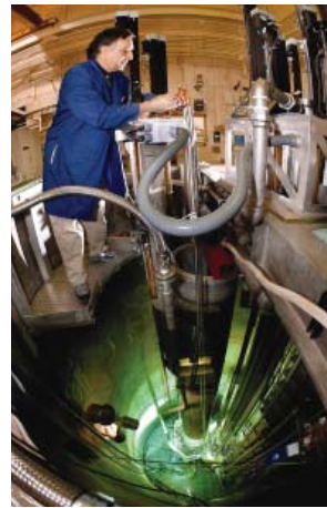
Reactor Operator Checks Equipment on the Annular Core Research Reactor, Which Sits at the Bottom of a 30-Foot-Deep Open Pool
