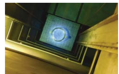
A Cobalt-60 Source Fixture Gives Off Cherenkov Radiation at the Bottom of the Gamma Irradiation Facility Storage Pool
